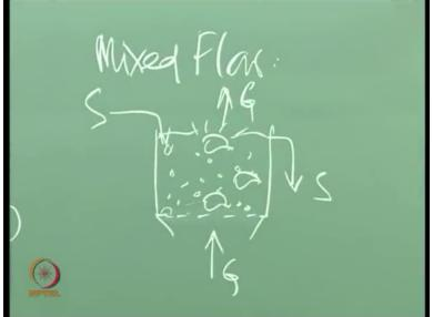
Again what is conceptually happening, I have the mixed flow like a fluidized bed and continuously mixed flow we have, okay. That is the distributor, this is the gas. We have the solid particles to start with uniform first then we have the bubbles and all that here bubble breaking small bubble. Okay. So, solids continuously coming, gas continuously going, yeah, okay.
