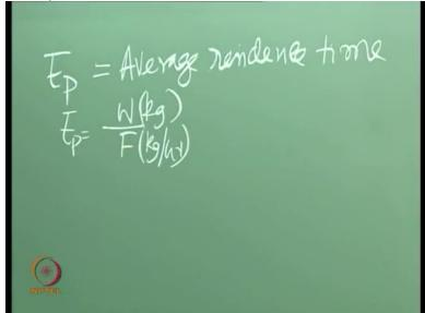
But the difference is that t is replaced by t bar p, where t bar p is, yeah, Average Residence Time, which is also defined as t bar p equal to W by F. W is holdup kg and this is mass flow rate kg per hour or kg per second whatever unit, okay. That is what is t bar p. For Tau bar p also, I am sorry, for t bar m also same equation W by F, okay, good.
