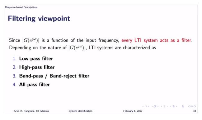
All these names are given based on how the amplitude ratio looks like as a function of omega. What kind of a filter is pure delay? All pass. It allows all frequencies to go through without any preferential treatment. Correct? So you should be familiar with all of this.
