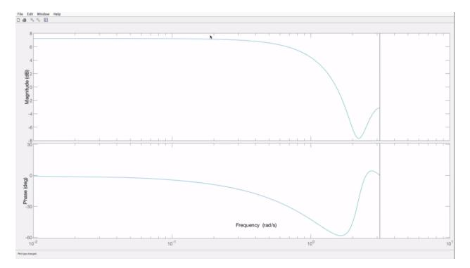
So, on the top you have amplitude ratio. It's not exactly amplitude ratio, you see something of that magnitude which is in decibels. Decibel is 20 times log 10 of AR. So it is not exactly plotting AR of omega. It's plotting 20 times log 10 AR. And this 20 log 10 AR has units of decibels in honor of Alexander Graham Bell. And we talk of always intensities and so on in terms of decibels. And phase is here plotted in terms of degrees not in terms of radians.
