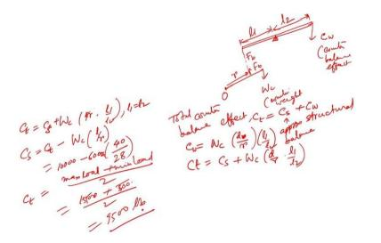
Next, let's consider another problem taken from Kermit Brown's book. The pumping system has the following buoyant weight of the rod:  $W_2 = 10,000$  pounds. Positive weight refers to the importance of the rod when it's immersed in water during pumping. It accounts for the buoyancy effect. Given that the fluid weighs 4,000 pounds, you must calculate the counterbalance (CB).
