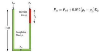
Now, let's discuss how the unloading process occurs, as described in Nguyen's book. Initially, imagine the entire wellbore: there is tubing, casing, and the entire space is filled with your completion fluid, which is a high-density liquid. Your hydrostatic column gradient will look like this, and there's a depth (D). For this example, let's assume there are 3 valves: V1, V2, and V3.
