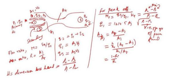
For peak efficiency (Mp), the mass ratio (Mp) can be calculated as  $Q_3 / Q_1$ , and the dimensionless head (Hp) is given by  $P_2 - P_3 / P_1 - P_2$ . The formula for  $Q_1$  is 1214.5 Aj  $\sqrt{(P_1 - P_3)} / \gamma$ , where  $\gamma$  is the density or specific gravity of the power fluid. These values are given in psi, with  $P_1$ ,  $P_2$ , and  $P_3$  all in psi as well.
