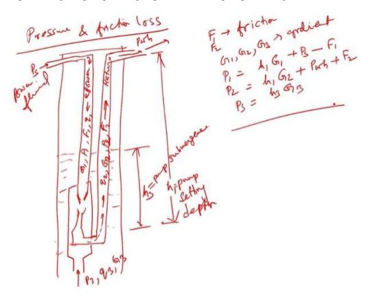
The fluid is served because of the nozzle created, allowing fluid to enter and move through the return channel. It returns as fluid enters the power fluid. We consider frictional pressure drop for  $F_1$ ,  $F_2$ , and  $F_3$ . For  $F_3$ , we assume there is no friction on the suction side, and we ignore the frictional pressure drop due to lower velocity.
