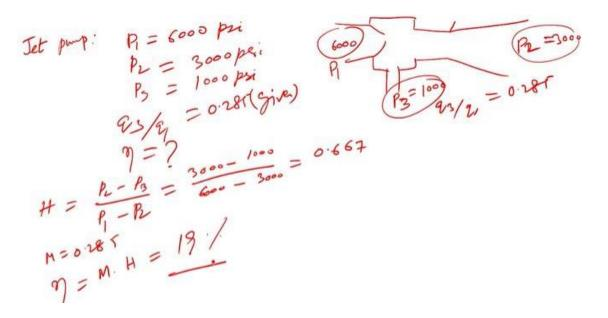
This problem illustrates how you can modify the given data to solve for different parameters, such as  $P_1$ ,  $P_2$ , or flow rates. Charts like the one presented earlier can also be employed to perform these calculations effectively. The information provided on the chart can be a valuable resource for problem-solving.
