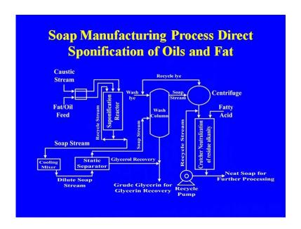
This is the actually, the flow diagram for making of the soap and we will discuss easy stage in detail. But you see the first this caustic soda and the fat and oil that is going to the saponification reactor, where the saponification is taking place and the after the saponification, here this is the saponification reactor where the saponification taking place. Then after that starts two steams; one is for the separation of the glycerine purification of the glycerine after settling.
