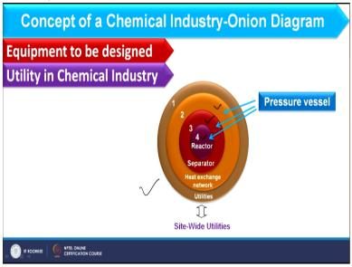
So here you see this is again the Onion diagram, different layers I have already discussed, and as I need to design the pressure vessel, through this pressure vessel we can design reactor, we can design separator, we can design heat exchangers. So this is the main reason of this course that once you study this course you can contribute in these three layers in the Onion diagram okay.
