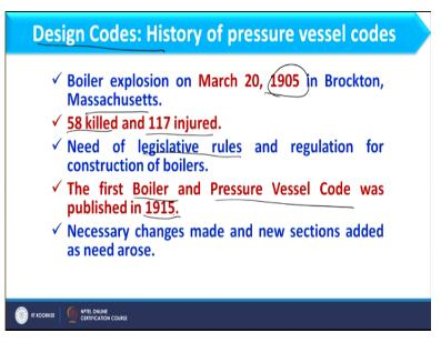
After this huge massive loss, there was a need to have some legislative rules and regulation for construction of boilers okay. So after that incident government has thought to provide some of the guidelines, so that those guidelines can be followed for design of boiler, okay. So first boiler as well as pressure vessel code was published in 1915. So first code was at the year in 1915 and after that as changes arouse and different corrections are made in that code okay.
