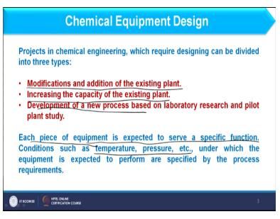
So the first part is modification and addition of existing plant. To make you understand this point, for example if I am considering one industry where obsolete technology is used, and at that place if you want to carry out the process through modern technology. It means some modification will be required, may be some new equipment or may be enhancement in the existing equipment will be required. So in that case or at that stage, mechanical design will play its role.
