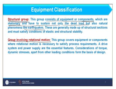
So second group in this classification is the structural group okay. So this group consists of equipment or component, which are stationary and have to sustain not only the dead load, but also natural phenomenon like earthquake okay. So what is this structural group. Structural group basically maintains the shape of the equipment. For example, if I am having a cylindrical equipment, throughout the life of plant, let us say it is 10 years or 15 years that shape should not deform okay.
