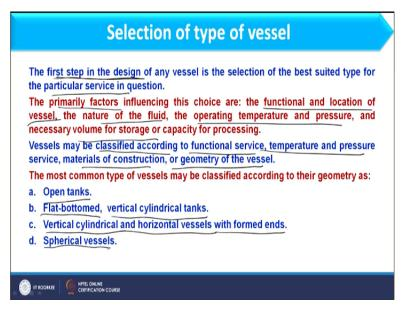
So the first step in design of any vessel is the selection of best suited type of vessel for a particular service in question. So according to the service, need to select proper vessel first of all and then we will design that particular or that proper vessel okay. So on what parameter that selection depends. First of all I need to select, so I have to see the parameters.
