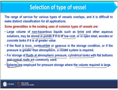
So those guidelines are, if you see, here I am having large volume of nonhazardous liquid such as brine and other aqueous solution may be stored in the ponds if it is of low cost. So that selection depends on the cost also, that is very important factor. If I need to store or operate very low cost fluid, so obviously for that purpose we can use open tank, where weather condition will not affect significantly okay.
