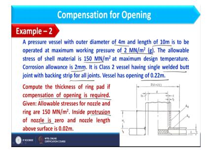
And here I am having second example, through which you will have more idea how to carry out compensation for opening. So in this diagram pressure vessel with outer diameter of 4 meter and length 10 meter is considered. And it is operated at maximum working pressure of 2 meganewton per meter square, allowable stress is 150 and corrosion is 2 mm, and this is again class 2 vessel with single welded butt joint with backing strip.
