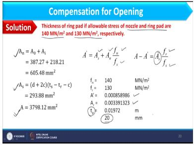
So we have to find thickness of ring pad if allowable stress of nozzle and ring pad are 140 meganewton per meter square and 130 meganewton per meter square respectively; however, for shell allowable stress value is given as 150 meganewton per meter square.
