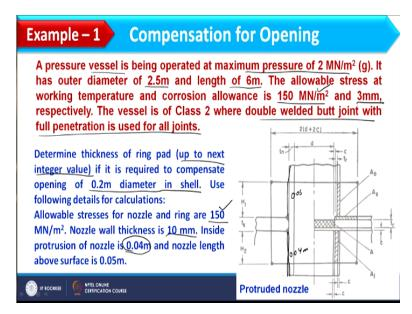
In this example, a pressure vessel we are considering which is operated at maximum pressure of 2 meganewton per meter square in gauge, outer diameter is 2.5, and length of shell is 6 meter, allowable stress at design temperature and corrosion allowance is 150 meganewton per meter square, and 3 mm.
