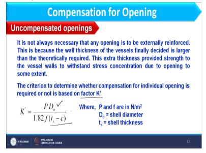
So what is K dash, K dash is basically defined by this expression, where K dash is equal to P D o/1.82 f t s – C, P is basically the design pressure, f is allowable stress, D o outer diameter of shell or where I am preparing that opening, t s is the standard thickness of shell or the part where I am creating the opening and C is the corrosion allowance. So based on this expression, first of
