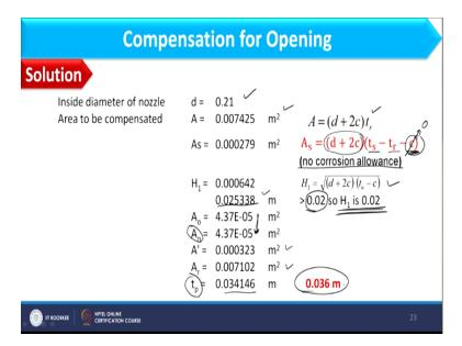
So here you can see this is the value of D 0.21. Area to be compensated, it will be calculated by D + 2 c \* t r, so using the values of different parameters I can calculate A, which is coming out as 0.007425. A s will be computed using the expression as D + 2 c \* t s - t r - c. Now in this case, t s is 36 and t r is 34.69 and c we have not added in this standard thickness. So in that case while computing A s value, we will not consider corrosion. So in that case this value would be equal to 0.
