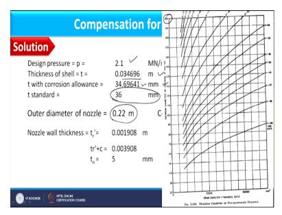
So up to 2 meter value we can see whether compensation is required or not through this graph. However, beyond this we should compensate and therefore in this case without computing I can say that compensation must be required.
