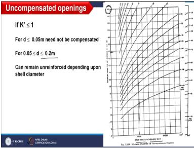
Now what happens, reinforcement is basically based on the diameter of component where opening is made. So for example if I am preparing opening in shell, so that would be the drum diameter, it means the shell diameter into thickness. So that thickness is basically standard thickness. So diameter as well as thickness I have to consider in mm and whatever value I am finding over here okay. Whatever value I am getting on X-axis corresponding to that value and
