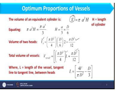
So Pi a 2 \* H, where H is the height of the cylinder that we have considered. Now, this volume would be volume of dome section, which we have just derived. So that Pi a 2 H will be equated to Pi a 3/3. And after resolving this, we can find H as a/3 and then a is basically D/2, so in terms of diameter it is D/6. So H we can represent in terms of diameter.
