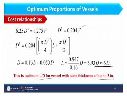
So putting this function to 0 we can have 6.25 D 3 = 1.275 V. So from this expression we can extract D 3 which is equal to 0.204 V and this V expression I already know as the volume of cylinder plus twice the volume of head as we have seen earlier. So that expression of V we can put over here. So D 3 will become 0.204 (Pi D 2/4L + Pi D 3/12), okay.
