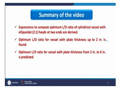
And here I am having summary of this video and it goes as expressions to compute optimum L/D ratio of cylindrical vessel with ellipsoidal heads where major and minor excess ratio is 2:1 at two ends are derived. Then optimum L/D ratio for vessel with plate thickness up to 2 inches is found and finally optimum L/D ratio for vessel with plate thickness from 2 inches to 6 inches is predicted. That is all for now, thank you.
