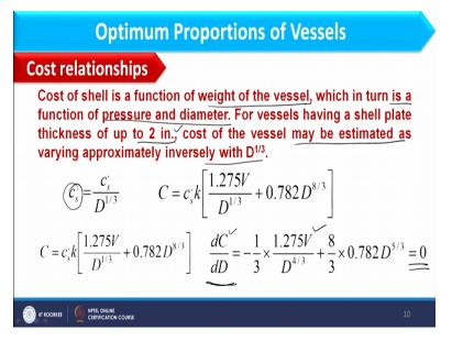
Now, further we will consider cost of shell as a function of operating condition, okay. In that case, cost of shell is a function of weight of the vessel we have already considered, which in turn is a function of pressure and diameter, okay. Now why it is function of a pressure because based on pressure we can find what should be the thickness of the vessel.
