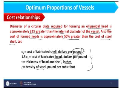
Now we have the cost relationships. Diameter of a circular plate required for forming an ellipsoidal head is approximately 22% greater than the internal diameter of the vessel. What is the meaning of this. If I am having internal diameter of the vessel is D, it means the plate through which ellipsoidal head will be prepared that would be 22% higher than the diameter of the vessel, so it would be 1.22D.
