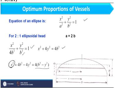
So, in this case as I am considering ellipsoidal head I will use equation of ellipse, which is x 2/a 2 + y 2/b 2 = 1. If I am having 2:1 ellipsoidal head, a should be 2 and b should be 1, so a should
