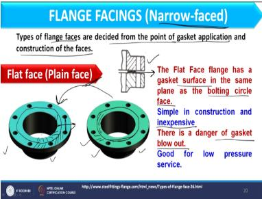
Flange face we are considering and here I am considering only narrow-faced. These flange faces are decided from the point of gasket application and construction of the faces. So here we are basically discussing different types of facing related to narrow-faced and narrow-faced you have understood that whatever gasket I am placing that gasket is lined within the bolt circle and that you cannot see from outside.
