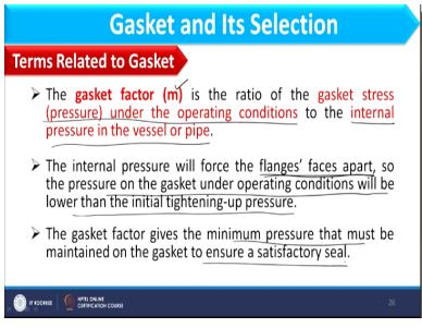
So one term I have considered as minimum seating stress, next term I am having is the gasket factor, and that gasket factor is denoted by m and it is the ratio of gasket stress under operating condition, okay. Two the internal pressure in the vessel or pipe. So this gasket factor is basically the ratio of gasket stress under operating condition. What is the meaning of this, that when operation is going on the joint should be tight enough, okay.
