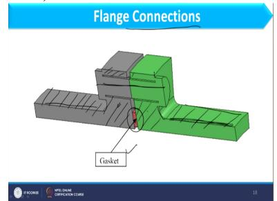
Now, if you focus on this particular figure it is basically speaking about flange connection. Now, here you see this section, what is this section if you are able to understand you can identify that this is the part of shell or the head or wherever that flange is connected, okay. So let us assume that this is the part of shell, okay. In the similar line this will be the part of shell. As we have discussed in the previous lecture that usually flanges are available in pairs, okay.
