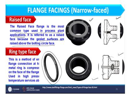
Second face in this category is the raised face and which can be considered or which can be defined as raised face flange is most common type used in the process plant application. So this is most common type. It is referred to as a raised face because the gasket surfaces are raised above the bolting circle face. Now what is the meaning of this that you can better understand from this image. Here we have two flanges or that is the pair of flange.
