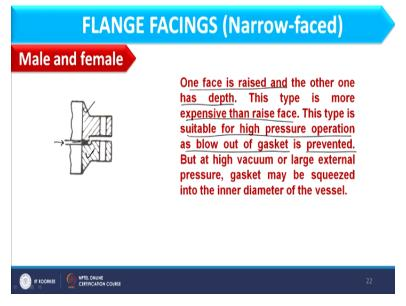
Next flange I am having is male and female type, how it is working and how it looks like, let us discuss that. So in this case one face is raised and other face has depth, okay. So basically this has different type of assembly where one has the raised surface another has deep construction or deep section, okay. So that raised face will lie within the deep section and therefore gasket is placed between the two faces.
