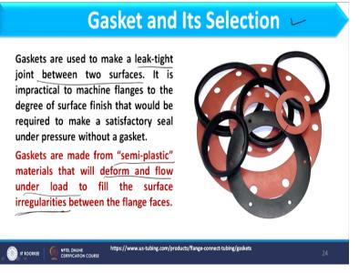
Now we have gasket and its selection. Gaskets are used to make leak-tight joint between two surfaces. So that we have discussed earlier also that whatever force I apply, whatever load we apply on two faces of metal, leak proof connection cannot be made, some irregularity or some opening may be there, which can be completely avoided by placing the gasket. So what is the basic role of gasket.
