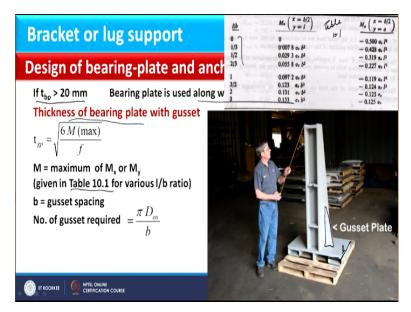
Further if bearing plate thickness is greater than 20 mm, bearing plate is used along with gusset plates okay. So here further we will use the gussets. So if you see this image, here basically this is the support, this is the column, and this is basically the bearing plate where this distance is given as l. So DO you can consider as outer diameter of shell because this will be aligned to shell okay. And if you see in this image, this particular section is called as gusset plates okay.
