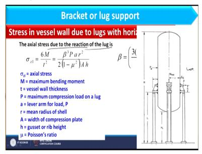
Now first of all you should understand this that once I am having the vessel and below we have the support, this vessel will put compressive load to the support okay. And further support will also react towards the shell because it will try to react towards the shell and because this vessel is acting downward that support will act upward, but direction would be axial only or longitudinal only.
