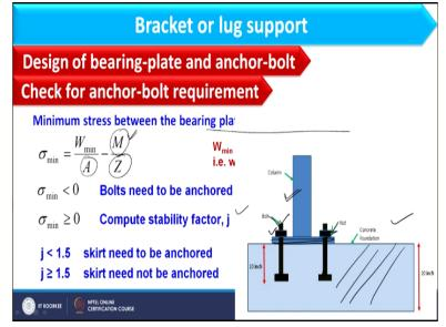
For that purpose minimum stress between bearing plate and concrete foundation should be computed using this expression, where sigma minimum is equal to W minimum/A-M/Z. Now why I am considering the minimum stress because when I am considering stability of the vessel as well as support the support will be most stable when it has the maximum load over this okay. It will not allow this to overturn.
