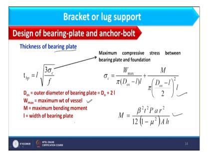
So thickness of bearing plate can be computed by this expression where t bp is equal to 1 root over 3 sigma c/f and sigma c is maximum compressive stress between bearing plate and foundation, which is given by this expression, where W max is the maximum possible load divided by Pi D OS - 1 \* 1 + M/this expression okay. So here you see D OS is the outer diameter of bearing plate that is D O outer diameter usually we can consider this as outer diameter of shell plus 21 okay.
