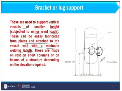
So here we have bracket and lug support. If you consider this is basically the vessel, okay, which is denoted as a over here and this particular assembly, which is denoted as b, this particular assembly is called as bracket or lug, and this c part is basically called as column, on which this bracket sits. So bracket and lug supports are used to support vertical vessel of smaller height. Smaller height means, which is subjected to minor wind loads.
