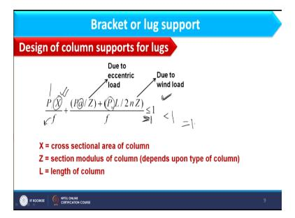
Here P/X/f + (P a/Z + P w L/2 n Z)/f, which is equal to or less than 1 okay. So this P if you consider this P is the total load on each lug that we have discussed earlier. X is the cross sectional area of the column okay, f is the allowable stress of column, and P is whatever we have discussed that is load on each lug, a is the arm that we have seen in the last slide divided by Z, Z is basically the modulus of this structure.
