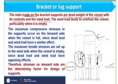
Now if you focus on this particular figure, here this is the vertical vessel where bracket support is attached and wind pressure is coming from this side as it is shown over here. So this is basically windward side. And here we have the leeward side where wind will try to turn. Now as we have discussed that there are two loads, first is due to dead load and second is due to wind load okay. Now once I am considering that dead load in this figure.
