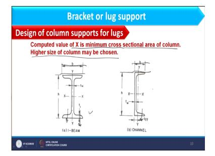
So as it is the minimum possible cross sectional area of the column higher size of column may be chosen okay. So we have calculated minimum cross sectional area. We will refer the standard and see whatever area available above than this that we can choose as a right column for the bracket to rest. So from where I will get that standard. So as far as columns are concerned we have definite shape for this like high beam channel etcetera.
