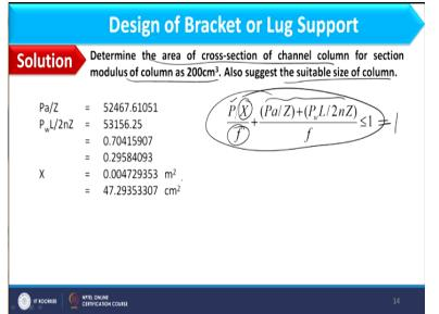
Next step I am having is to determine the area of cross section of the channel column for sectional modulus of 200 cm cube okay. And we need to suggest the suitable column for the bracket okay. So this is the expression to calculate the cross sectional area of column, where X is the cross sectional area of column. All these parameters we have already discussed in the last lecture okay.
