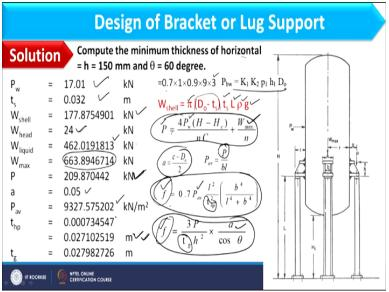
Now I need to find out thickness of horizontal as well as gusset plates. For that case if you consider this is the expression to find out thickness of horizontal plate okay. And to compute this I need to calculate P av first and for calculation of P av I need to find out total load on each lug okay and that is given by this particular expression.
