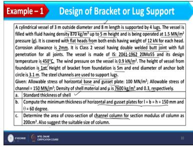
Now we will see few examples for support design. So here I am having example 1 and in this example the cylindrical vessel of 3 meter outside diameter and 8 meter length is supported by 4 lugs, so this example is basically related to bracket or lug support, which we have discussed in last lecture. So the vessel is filled with the liquid or fluid having density 870 kg per meter cube up to 5 meter height and is being operated at 1.5 meganewton per meter square in gauge.
