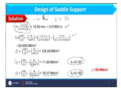
So considering these movements we will calculate all stresses, but these stresses will also require thickness of shell and therefore we can compute minimum thickness of shell using usual expression and here if you remember 1.2 meter R is given, which is internal radius, so internal diameter would be 2.4 okay. So that we have used over here and therefore this minus sign appears and minimum thickness comes as 16.92 mm.
