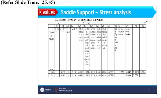
Here we have values of constant for saddle support. So here we have contact angle that is 120 is the minimum angle and 122 and we have long table which I will show further. And here we have K 1, K 2 for different conditions like A is less than R/2 or other condition and then K 3 when shell is stiffened by end of the vessel and we have other conditions also. And similarly K 5, K 6, K 7, K 8 and K 9. So here you see values are available at 120 and 122.
