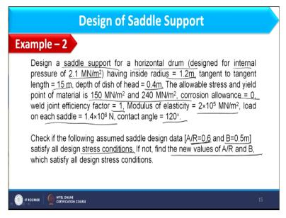
Now here I am having second example, which is on design of saddle and in this example I need to design a saddle support for horizontal drum, which is designed for internal pressure 2.1 meganewton per meter square, internal radius 1.2 meter is given, tangent to tangent length is 15, depth of the dish of head that is H as 0.4 meter is given, allowable stress yield point of the material are given as this.
