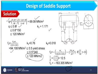
So considering K 3 as this we can find out q, which is coming out as this and this should be lower than 0.8 \* f, so it is well satisfying the condition. Next we have the f3 value and f3 will be given as K 5 W 1/t (B + 10t) and K 5 you can see as 0.76 and here you can see K 5 as 0.76 from this table corresponding to 120 degree, and considering these points K 3 comes as 94.108, which is well satisfying the condition that is it is less than 120 meganewton per meter square.
