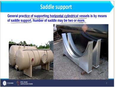
So general practice of supporting horizontal cylindrical vessel is by means of saddle support and number of support or number of saddle may be two or more. So basically this saddle support is used for horizontal vessels and how it looks like that we can see from these images. So if you see this image here we have the horizontal cylindrical vessel okay, different sections you can
