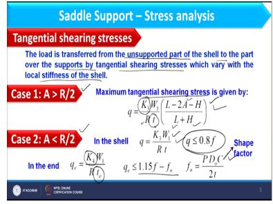
Now load is transferred from unsupported part of the shell to part over the supports by tangential shearing stress that we have discussed already, which vary with the local stiffness of shell. What is the meaning of that local stiffness. For example, if I am providing some structural support to the cylinder or to the vessel the load will be transferred or the circumferential stress will also be transferred to that structure okay.
