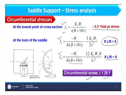
So at the support at lowest point of cross section we can calculate stress as f3, which is equal to K 5 W 1/t (B+ 10t) and that should be equal to 0.5 into yield point stress. And at the horn of the saddle, what is that at horn of the saddle, where edge of horn is appearing in shell, so that is basically the end of support in shell. So there we have circumferential stress as f4, which is equal to -W 1/4t (B + 10t) - 3 K 6 W 1/2t 2 and this expression we will use if L/R is greater than 8.
