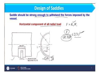
So till now we have discussed stresses which are falling in shell due to shell. Now we will discuss design of saddle because whatever stresses are occurring in shell or what as or whatever forces are apply in metal sheet of vessel or the weight of vessel itself that should be withstand by the support. So support should also be strong enough to bear all these loads. So for that purpose we have to satisfy the design equation which is related to saddle. So let us discuss that.
