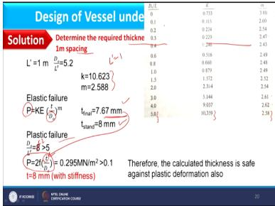
So when stiffeners are located at 1 meter spacing, it means that effective length would be 1 meter in this case. So D O/L dash comes as 5.2 okay. And here I am having the elastic failure and here corresponding to D O/L dash = 5.2, I can find out value of K as well as m from this table and here you see value is available slightly higher than this. So it is very close to 5, so here we can extrapolate the values to know the values of K and m. And K we can find out as 10.623 and m as 2.588.
