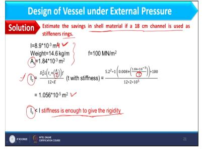
And now I need to estimate the savings in shell material if 18 cm channel is used as stiffening ring. For this channel, value of moment of inertia is given as 8.9 times power -3, here we have meter power 4 okay, and weight of stiffener is 14.6 kg per meter, f is given like this and here we have the sectional area A S, which is 1.8 times power -3 meter square. Considering all these values we will find out I C, which is basically the moment of inertia for the structure with circumferential ring.
