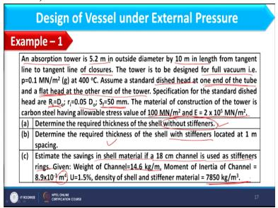
So this example says that an absorption column of 5.2 meter outside diameter and 10 meter length from tangent to tangent line of closures. So I guess you understand what is the meaning of tangent to tangent line that is nothing but the length of the shell. This tower is to be designed for full vacuum that is 0.1 meganewton per meter square at 400 degree Celsius. Assume a standard dished head at one end of the tube or tower and a flat head at another end of the tower.
