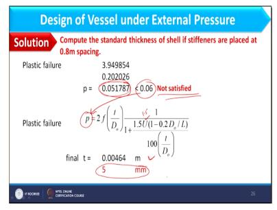
And then we will go for plastic failure condition. This gives me the pressure for plastic failure considering 4.27 mm thickness, and if you see this is less than the design pressure, design pressure was 0.06 and in plastic failure condition it is coming lesser okay. So it will not satisfy the condition. So for that purpose we will consider p as 0.06 and which will be given by this whole expression where U should be 1.5 as we have discussed earlier.
