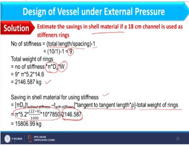
And then I have to find out saving in the shell material. So as far as saving in shell material is concerned how I can calculate this because when I am not using stiffeners the thickness was 22 mm. And when I am using stiffeners thickness becomes 8 mm, but at the same time I am investing in stiffeners also okay. So first of all I have to find out number of stiffeners and how much material will be required for these stiffeners.
