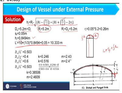
And as you have seen the example that in this vessel one side have flat head and another side has domed section or form section. As you can see from this diagram, here we have this is shell and this is form section. Now this height of form section is hi and to consider this domed section in effective length I am considering one-third of hi here okay. So first of all I have to determine what is hi, so hi you can find out through this expression.
