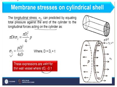
Now, another expression I am considering longitudinal stress that is sigma 2. Here sigma 2 basically represents longitudinal stress and that would be balanced by the forces which are acting on the cylinder in longitudinal direction, okay. So, if you consider this particular image, here we have sigma 2. Sigma 2 will be applicable in this region, okay, in this whole region sigma 2 will be active. So, that sigma would be what, that pressure into acting area. Acting area will be this area.
