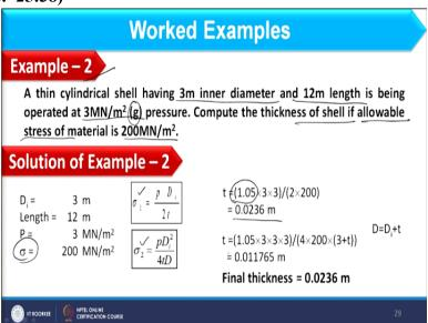
So here I am having example 2, where a thin cylindrical shell having 3 metre inner diameter and 12 metre length is being operated at 3 mega N/m square G. what is this G, G is nothing but the gauge. So, pressure is given in gauge. Why I am considering pressure in gauge that we will
