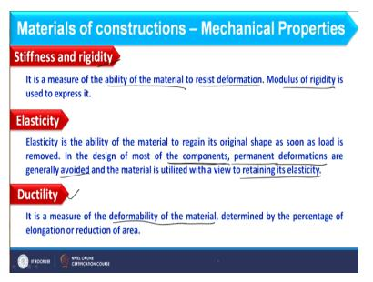
Second property is stiffening and rigidity. It is a measure of the ability of the material to resist deformation and modulus of rigidity is used to express this property. And next, I am having elasticity. Elasticity you understand that when we apply stress to a particular object, it deforms. When we remove that load or stress, that material will regain its original shape, so that we can call as elasticity of the material.
