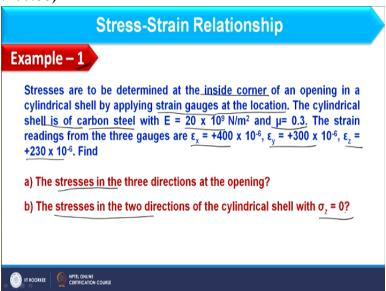
And here I am having example 1, and it states that the stresses are to be determined at the inside corner of an opening in a cylindrical shell by applying a strain gauge at the location. So in this problem, a cylindrical shell is considered, where an opening is made and due to this opening, whatever strains are generated that are measured through strain gauge, which is a instrument to find out the strain at a particular location.
