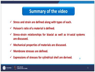
Now, we have the summary of the video and this summary is combinedly written for lecture 2 as well as lecture 3, and here stress and strain are defined along with types of each, Poisson's ratio of a material is defined, stress and strain relationship for biaxial as well as triaxial system are discussed, and mechanical properties of material are discussed. Membrane stresses are defined and expression of membrane stresses for cylindrical shell are derived.
