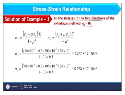
In second part, we need to find out stresses in two directions of cylindrical shell where sigma Z is equal to 0. So here I am having the relation of sigma X as well as sigma Y as a function of epsilon X and epsilon Y. This is biaxial system. These equations we have already derived and while putting the value of strain E and Mu, we can have sigma X as well as sigma Y, okay. So, sigma X, it is simply the expression based, not complicated solution is required for that.
