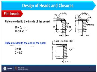
Now, further, we have another attachment or another connection, and that is plates welded to the inside of the vessel, so how it looks like? Here, I am having this shell and inside this shell head is attached. If you consider the previous diagram, there head is attached to the shell through butt welding. I hope you remember different types of welding which we have discussed in lecture 4 of week 1 in weld joint efficiency factor, okay.
