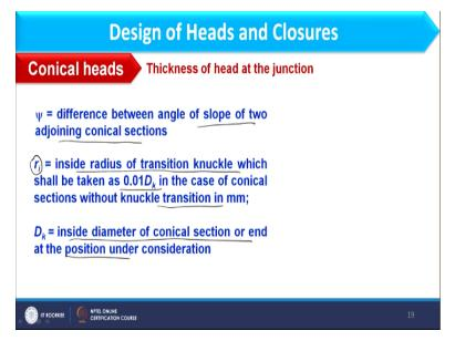
So, here you see, Si I am having, Si is the difference between angle of slope of two adjoining conical sections and I have already discussed why the Si is there. Si and alpha both angles are there, but in some cases these two angles are different. Therefore, we have used different notation for these two. How it looks different, that we will discuss.
