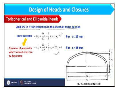
So, once I am having this, we will calculate the blank diameter. What is blank diameter? It is the diameter of plate with which form Ls can be fabricated. So, if I am having this ellipsoidal head, the diameter means the diameter of this whole section, whole plate through which this ellipsoidal head is prepared, so that would be equal to  $D \circ + D \circ /42 + 2/3$  R i +2 SF. SF you can understand, SF is basically this straight part, which is beyond the curved section.
