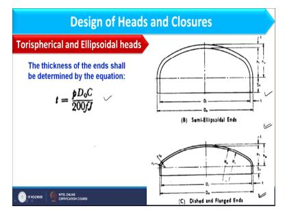
Now we will discuss design of torispherical heads as well as ellipsoidal heads. So, these heads are basically coming under dished or formed heads. So, you see this image, where this figure is of torispherical head and this figure is of ellipsoidal heads, so both heads are basically dished heads, however, in ellipsoidal heads, we have more curved part in comparison to torispherical heads and these two heads are designed using same expression as these are dished heads.
