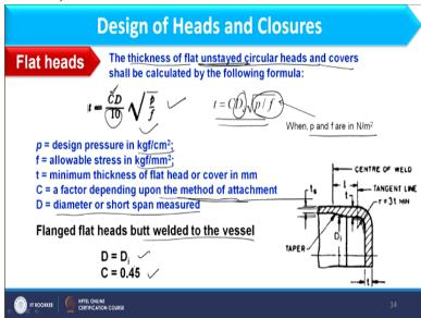
Now, in this case, we will calculate thickness of flat unstayed circular heads and curves, okay? So, you see here we have one term that is unstayed circular heads, what is the meaning of unstayed circular head? To illustrate this or to make you understand, I am taking the example of this glass, now if you see this glass, this is open part of this glass where I need to cover, so what is the meaning of unstayed. To understand this, let us first discuss what is stayed.
