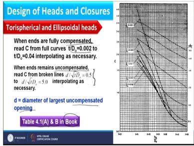
And once H e will be known, in this figure, you can make a line, okay. Let us say H e is 0.2, so corresponding to 0.2 you can make a line and how you need to find out value of C is, when ends are fully compensated, read C from full curves that is T/D o 0.002 to 0.00 that is T/D oequal to 0.002 to T/D o 0.04 and we can make interpolation also.
