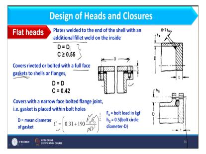
Now next connection I am having is plate welded to the end of the shell with additional fillet weld on inside, okay. So, this is noting but the previous diagram only. At the end of shell, head is attached with fillet. So, you can see the value of C and D would be D in this case. Now, next I am having is curves R iveted or bolted with full face gasket to shells or flanges.
