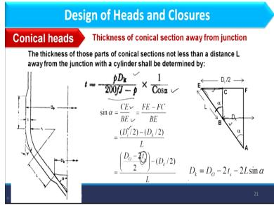
So to calculate thickness of that part, we have this expression as T = PD k/200 f J - P 1/Cos alpha. Here, P is the design pressure, why 200 is there, I hope you have idea this till now, because P and f are different units, J is the joint efficiency factor.
