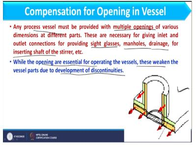
So, that opening, let us say it is used for feed inlet, feed outlet or we may use that for sight glass, so for all this purpose, we need to create some opening in a vessel, so that opening usually circular or that may be rectangular. So, when we have any opening, it means we are cutting a particular section in a regular sheet.
