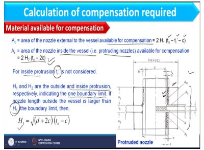
So, if you consider this image, what is A o, A o is basically area of additional material available in nozzle above the vessel surface, okay. So, this is basically the A o. In the similar line, A i is the area of additional material available inside the vessel in the nozzle. So, A o and A i we will calculate and for that purpose, you should understand that as far as total length is concerned, we have considered H 1 as well as H 2.
