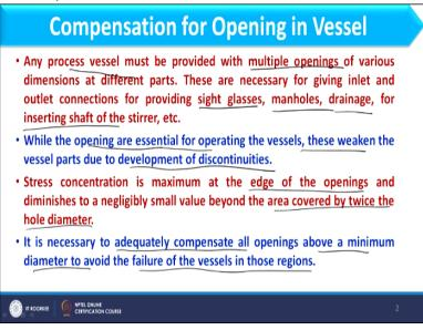
So, stress concentration is maximum at the edge of the opening and diminishes to negligibly small value beyond the area covered by twice the whole diameter, okay. What is the meaning of this? Let's have example of that cloth only, when I am having the hole over here, okay, and
