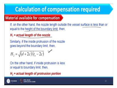
On the other hand, nozzle length outside the vessel surface is less than or equal to height of the boundary limit, then H1 would be the actual length of the nozzle. So, what is the meaning of this? That we will calculate H1 and then we will compare that H1 with the length of nozzle outside.
