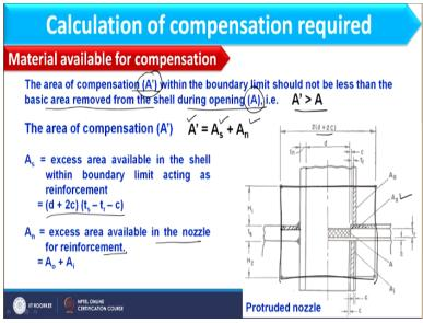
So, material available for compensation is the area of compensation that is A dash within the boundary limit should not be less than the basic area removed from the shell during the opening. It means A is basically the area which needs to compensate and A dash is basically area of additional material available for compensation. So, in no case, A dash should be less than A. Preferable condition would be when A dash would be greater than A.
