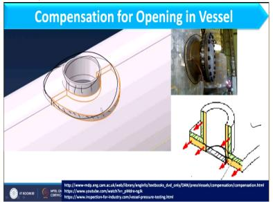
So, if you consider this example, here I am having the hole where I have put this nozzle and this is basically the compensation. So, if you observe this compensation, this is what, this is basically extra material we have placed around the nozzle, okay.
