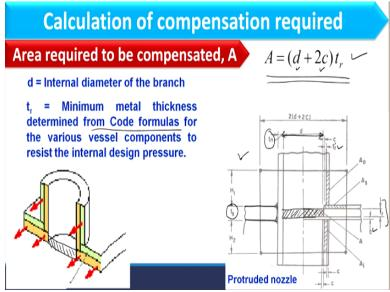
Now we will start calculation for compensation. It means whatever opening we have created, that we have to reinforce. So, how much area I need to provide for reinforcement. Until now you must have the idea that compensation or reinforcement whatever I am providing, that will be in terms of a ring. So, what should be the thickness of that ring pad. So all these calculations we will consider here. So, let's start this.
