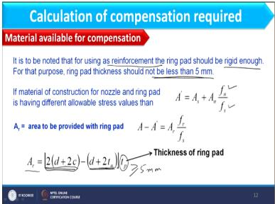
Now, it is to be noted that using as reinforcement that ring pad should be rigid enough. That rigidity I have to ensure and therefore ring pad thickness should not be less than 5 mm. If ring
