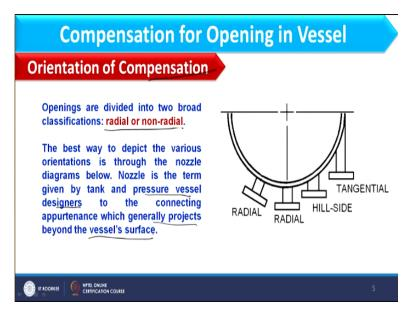
So, basically orientation of nozzle speaks about orientation of compensation because as I have to place the nozzle, accordingly I have to create the compensation, okay. So openings are divided into two broad classifications, radial and nonradial and the best way to predict the various orientation is through the nozzle diameter as shown over here and nozzle is the term given by tank and pressure vessel designers to the connecting pertinence which generally projects beyond the vessel surface.
