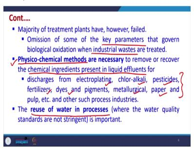
Majority of traditional treatment methods, if they have been applied for industrial wastewater, they have failed. And because these conventional treatment methods, they are not able to remove various other pollutants, which are present in these industrial wastewater and they are not able to remove. So, these pollutants remain in the water after treatment also.
