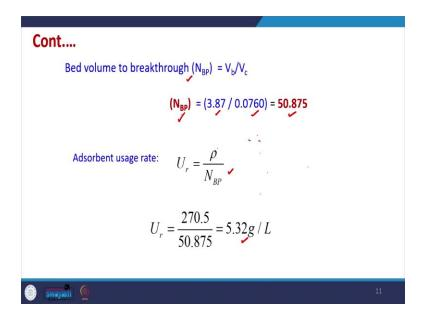
So, we can calculate some of the calculations, we can perform here like calculate the empty bed contact time for the furfural adsorption in a packed bed of bagasse's fly ash at given conditions. So, the concentration, suppose the initial concentration is 100 milligram per liter, flow rate is 0.02 liter per minute, bed height suppose is, we are carrying out this work only in lab scale.
