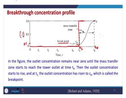
So, this is the breakthrough point that we have pointed out earlier, the breakthrough point, when the adsorbent reaches the characteristic limit, suppose this is 0.01. So, if it is reaches this condition that means after that the bed is not good enough and the water which is coming out, it contains the adsorbent up to a concentration which is not desirable. And after some time, there will be a point where the C by C0 value will reach 1.
