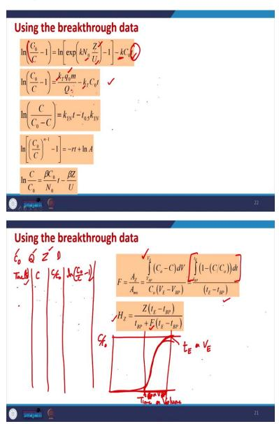
Similarly, we can use the same data. So, we have C by C0 versus time data. So, we can use convert that data into this form and take log of that and draw the curve with respect to time. So, if we can draw the curve and C0 since already it is known. So, slope of the curve will give k and
