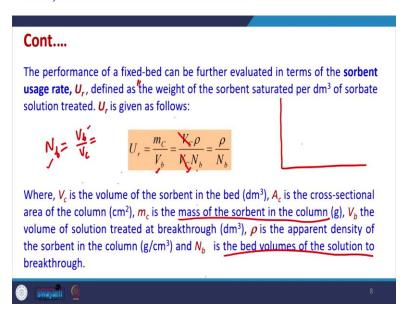
The performance of a fixed-bed can be further evaluated in terms of the sorbent usage rate,  $U_r$ , defined as the weight of the sorbent saturated per dm<sup>3</sup> of sorbate solution treated.  $U_r$  is given as follows:
