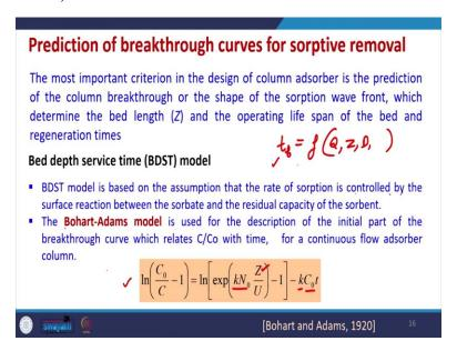
The Bohart-Adams model is used for the description of the initial part of the breakthrough curve which relates C/Co with time, for a continuous flow adsorber column:
