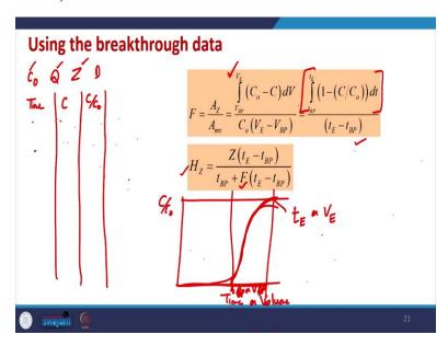
So, let us try to see. So, what we do is that in the lab scale, we perform some experiments, like where we have two, three different types of small beds, which may be there. And in the bed they may be of different diameter, we can keep different height also and we can certainly change the flow rates also. So, at any flow rate suppose, C0, where the flow, at one flow rate we have initial concentration is known and Z is also fixed and diameter is also fixed.
