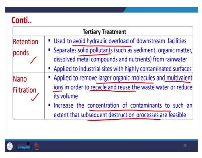
So, then we have tertiary treatment using retention, ponds nanofiltration. So, retention ponds can be used for avoiding hydraulic load one load of downstream facilities if you are going to use other treatment strategies and it can be used for separating solid pollutants from rainwater et cetera. Nanofiltration also removes large organic molecules and multivalent ions also. So, this this way, if we are able to remove this, we can use the recycle reuse the wastewater.
