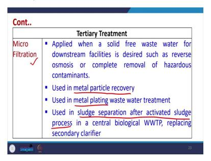
Each of these sections have been studied in detail you can go back and again see the lectures to better understand then we can have micro filtration technique, which is applied when a solid free wastewater for downstream facilities desired such as RO or complete removal of hazardous contaminants. So, in this case we have microfiltration can be used.
