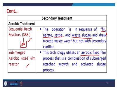
Now, the system is designed to be installed in two compartments where the first compartment provides majority of BOD removal and the second compartment polishes the BOD. So, this this is how it works. Then we have membrane bioreactors also they are being used to treat municipal as well as industrial wastewaters.
