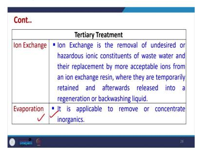
Now, in the last week we can go for removal or destruct most of the organic compounds using the evaporation technique. So, this is how we can use the evaporation technique.
