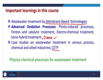
Then also we studied the wastewater treatment by membrane-based technologies, including the microfiltration, ultrafiltration, nanofiltration and RO. So, all these technologies we studied thereafter, we studied advanced oxidation processes and these included that like photocatalysis Fenton process, catalytic wastewater treatment, then electrochemical treatment or ozone treatment et cetera. And then the hybrid technologies also including the sono hybrid treatment techniques.
