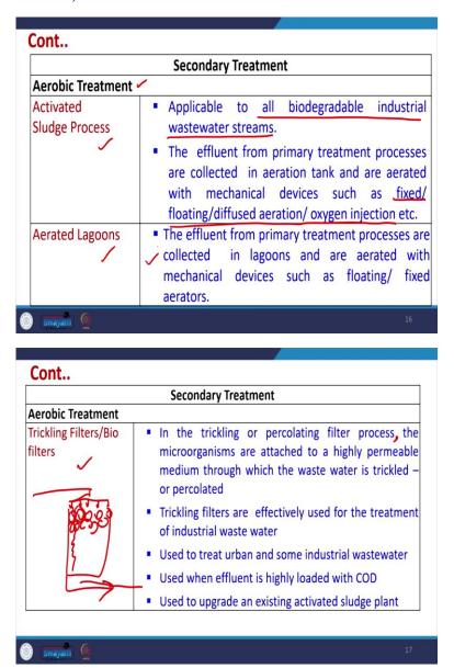
So, what are the still just for the knowledge there are two options one is called aerobic treatment another is called anaerobic treatment. So, within aerobic treatment activity sludge process, aerated lagoons, trickling filters et cetera are common techniques. So, any of these techniques can be used for biological treatment or secondary treatment. So, it is activated sludge processes the most common technique and it is applicable to all biological industrial wastewater streams.
