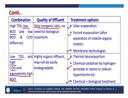
So, these are the strategies similarly, if high TDS, BOD and COD, BOD is low and the difference is also low. So, that means only inorganic salts no need for biological treatment we can go for solar evaporation, forced evaporation or membrane technologies, because the BOD is not there and the difference between BOD and COD is also less only in organics salts are present that means.
