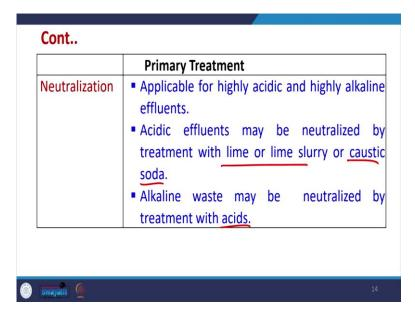
Now, in the primary treatment, some neutralization may be done depending upon whether we have highly acidic or highly alkaline effluent. The acidic effluent can be neutralized by
