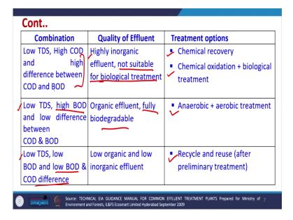
So, these are the general combination which are possible, again low TDS, high COD and high differences that means, there is a lot of difference between COD and BOD. So, that means the BOD value is very less. So, that means it is not suitable for biological treatment. Now, that means it has high inorganic content and we can go for chemical recovery or chemical oxidation plus linked in with amount of biological treatment.
