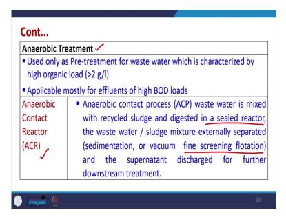
Now, going to anaerobic condition they are used as a pretreatment of wastewater which is characterized to have very high organic load. So, the idea is that if any wastewater is having very high organic load. So, why not use this high organic load to convert that into methane and other types of useful products. So, because of this if any wastewater contains very high organic load, we can go for anaerobic treatment and that can be done in anaerobic contact reactor.
