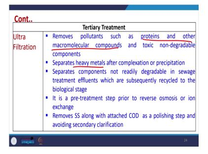
Then ultra-filtration so, all these are membrane-based technologies microfiltration, ultrafiltration, nanofiltration and RO. So, they remove pollutants such as proteins and other micro molecular compounds and toxic non-degradable compounds, they can separate heavy metals also after complexation of precipitation and this ultrafiltration can technique can be used as pre-treatment step also before RO.
