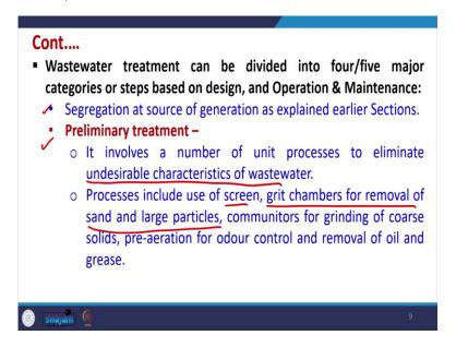
Now, wastewater treatment can be divided into 4 or 5 major categories or steps based upon design operation and maintenance that we have learned. So, we will try to understand this. So, first is preliminary treatment to segregation at source of generation has been earlier explained. So, this is very important and this helps in determining that which strategy has to be followed. Now, after that, there are different options one is preliminary treatment.
