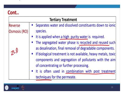
Then similarly RO units also based upon the same idea that they separate water and dissolved constituents down to ionic species, it is applied when a very high purity water is required. So, RO units are very common, the segregated water phases are recycled and reused. So, RO units are always used whenever we have to recycle and reuse the water in particular, suppose we have to use the water in highly pure form.
