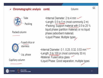
So, this is our packed weight column. Say if it is a packed weight, so, this is our tube, outside is our tube and then inside is we are having say these are packing materials. And in this case, the internal diameter of the tube is 2 to 4 mm and length is 0.5 to 5 m. Support material with 0.5 to 25% liquid phase. And liquid phase may be of multiple types.
