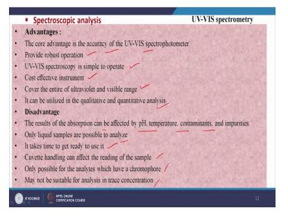
So, UV visible has some advantages as well as disadvantage. So, the core advantage is the accuracy of the UV visible spectrophotometer provide robust operation UV visible spectroscopy is simple to operate and cost effective instrument and cover the entire of ultraviolet and visible range. So, wide range of wavelength they can handle and it can be utilized in the quantitative and qualitative analysis.
