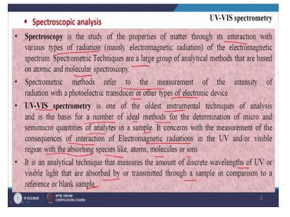
Now, we will see first UV visible spectrometry. So, spectroscopy is the study of the properties of matter through its interaction with various types of radiation, normally, electromagnetic radiation of the electromagnetic spectrum and spectrometry techniques are a large group of analytical methods that are based on atomic and molecular spectroscopy.
