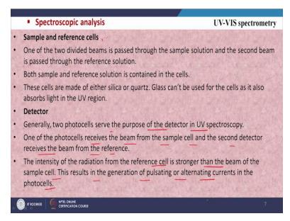
So, that will be your sample and reference cells two cells are needed. And if it is a double beam, then simultaneously the light two beams will be sent one through the sample and another to the reference and if it is a single beam, so, it will be sent once it will be sent to the sample and after that, it will be sent to the reference, not simultaneously. So, that way two different arrangements are there and then after that, we will detect, detector is necessary.
