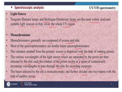
Now, if we see the different parts of the UV visible then one is that we have to send some light UV light. So, light source is needed, so tungsten filament lamps and hydrogen deuterium lamps are the most widely used and we have to send a monochromator. So, monochromator generally are composed of prisms and slits, we have to send one type of ray or wavelength we have to send. So, most of the spectrophotometers are double beams spectrophotometers.
