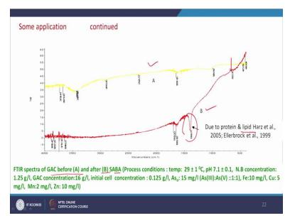
So, here it is, it is giving us two, this is A and this is B. So, A is nothing but FTIR spectra of GAC before and after SABA, that is simultaneously adsorption and bioaccumulation method. So, if we take say scale water samples and adsorption, then that will be only adsorption if we use microbes and the pollutants then also there will be biodegradations or in case of conservative pollutants like say arsenic though arsenic will not be degraded by the microorganisms it will be captured and stored.
