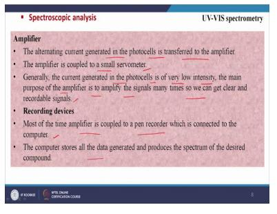
And then that amount of current which is generated that is not very high. So that has to be amplified, so amplifiers are used, the alternating current generated in the photo cells is transferred to the amplifier, the amplifier is coupled to a small servometer and generally the current degenerated in the photo cells is a very low intensity, the main purpose of the amplifier is to amplify the signals many times so we can get clear and recordable signal.
