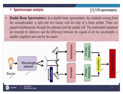
And this is for a double beam spectrometers. So, in this case, source wavelength selector wavelength selector is giving us two beam these two beams. So, these two beams are simultaneously it is one beam is going to the reference and another is going to the sample then this is we have photodetector here also photodetector so, then the difference is giving some signal and that is amplified and again it is going to output device.
