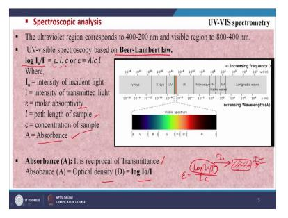
So, how does UV visible spectroscopy spectrometry works? It works on the principle of Beer-Lambert law, what is that principle? So, if we pass some radiation or UV light through a sample which is present here. So, when it will be passing through it, the some part of light or electromagnetic radiation will be absorbed and particularly in this case of UV, UV light will be absorbed and the intensity will be reduced.
