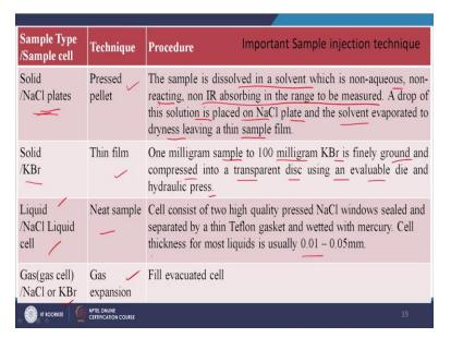
Like say, NaCl plates can be used or potassium bromide can be used for solid samples. So, if NaCl plates are used in that case, so the technique is called pressed pellets and one KBr the technique is thin film. So, in this in this in the first case for NaCl plates, the sample is dissolved in a solvent, which is non-aqueous and non-reacting, non IR absorbing in the range to be measured.
