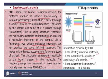
Then next is FTIR spectrometry that is Fourier transform infrared spectrometry and FTIR stands for Fourier transform infrared, the preferred method of infrared spectroscopy. In infrared spectroscopy IR radiation is passed through the sample unlike UV visible, in case of UV visible we pass UV visual range of monochromatic light, but here in FTIR we will be processing IR light.
