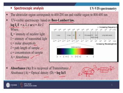
So, UV and visible the main difference is their wavelength, the monochromatic light which we are generating that wavelength the visible is high having more wavelength, as you mentioned here so the ultraviolet region corresponds to 400 to 500 nm and visible region. So, 400 to 800 nm is your wavelength.
