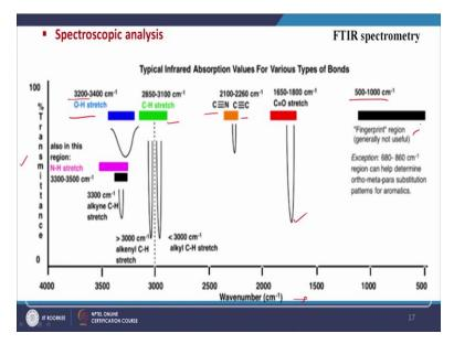
So, if we see this type of spectra we will get, so this is your percentage transmittance and this is our wave number. So, in this wave number we see we get different peak here due to transmittance. So, these two this range, it is CH stretch, OH stretching this to this is 3200 to 3400. Similarly, 2100 to 260 CN or C, triple C, CC triple bond. So, these are the different functional group as we were talking about. So, now if C double bond strength is responsible for these peak again.
