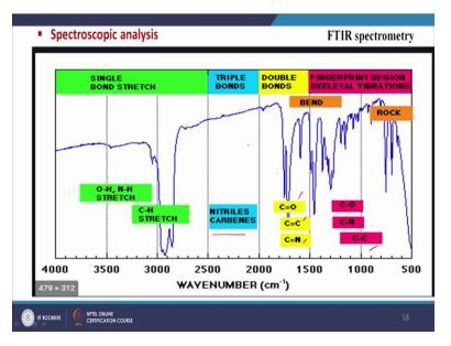
This is another example here also single bonds stretching triple bonds, double bond. So, the IR has low energy, so as I have mentioned it is absorbed by the molecules as for the different vibrations and rotations of the double and triple bond, so that way the different peaks are generated. So, this peak is CO, CC, CN, CO, CN, CC like this. So, nitrile if it is nitriles or carbons so, within this range we can get some peak.
