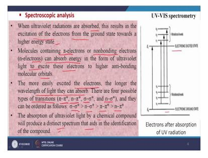
When ultraviolet radiation are absorbed, this results in the excitations of the electrons from the ground state towards a higher energy state. So, when we are sending some radiation, let us say UV radiation are visible also UV and visible UV is more powerful than the visible, then both are having some capacity to excite the external electron from their base to the excited state for example, here you see these are base position and these are excited position.
