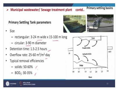
And primary settling basins or primary settling tank parameters the size normally 3 to 24 m wide and 15 to 100 m long, and that may be circular 3 to 90 m diameter, and detention time 1.5 to 2.5 hours, overflow rate 25 to 60 m<sup>3</sup>/ m<sup>2</sup>-day and typical removal efficiency solid 50 to 60 % and BOD<sub>5</sub>, 30 to 35 that is the primary settling basin.
