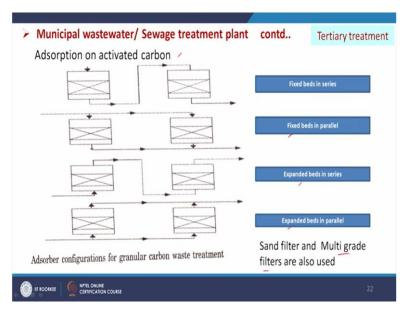
After that it the water is to be sent to the tertiary treatment, tertiary treatment is basically which is used in industry and wastewater treatment plant, domestic wastewater treatment plant that is carbon waste filters and sand waste or multigrade filters are used. So, as shown here adsorption on activated carbon, the very small amount of TDS or BOD which is available after the secondary treatment that can be further fine-tuned or can be removed here and these systems used as a polishing step.
