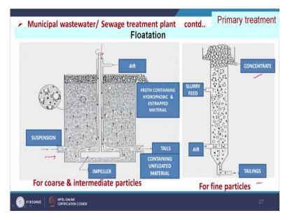
And we will see the flotation unit. So, floatation unit, our objective will be to remove the materials which are less dense so, that by the applications of air so, here we are providing air and here the suspension is coming, so air will be trying to make some layer at the surface of the particles and it will make more hydrophobicity, it will increase the hydrophobicity and it will help to rise the particles.
