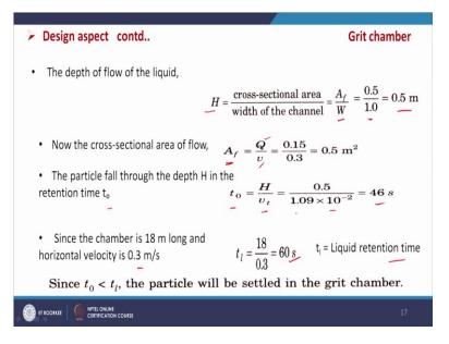
Now, the depth of flow of the liquid we have to calculate. So, if it is H and if we multiply the width of the channel then we will get the cross-sectional area. So, cross sectional area is the height \* width of the channel.
