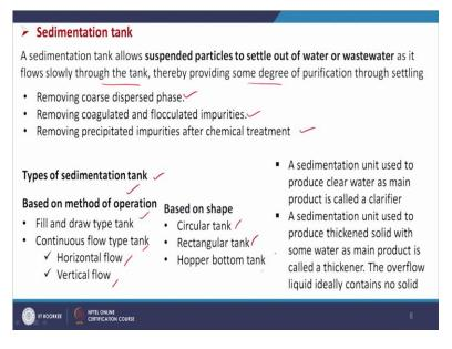
Then sedimentation tank. So, a sedimentation tank allows suspended particles to settle out of water or wastewater as it flows slowly through the tank thereby providing some degree of purification through the settling. And it helps to remove coarse dispersed phase, it helps to remove coagulated and flocculated impurities and removing precipitated impurities after chemical treatment. BOD can also be removed and TDS can also be removed.
