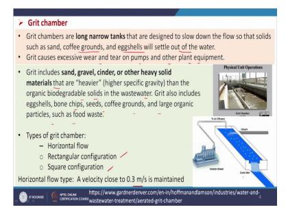
And now we will see the grit chamber. So, as you have seen the grit chambers are basically used to separate the heavier particles. So for that grit chambers are long narrow tanks that are designed to slow down the flow so, that solids such as sand, coffee grounds, and egg shells will settle out of the water.
