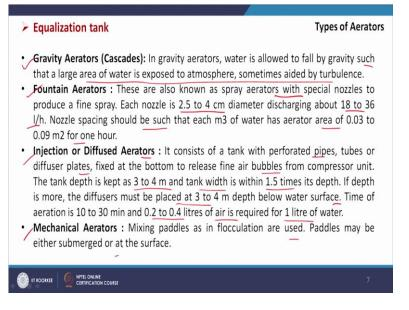
And then aerators, there are some aeration systems are available that is gravity aerators, fountain aerators, injections or diffused aerators, and mechanical aerators. So, in gravity aerators water is allowed to fall by gravity such that a large area of water is exposed to atmosphere sometimes aided by turbulence. So, water is falling under gravity and is coming in contact with the air or oxygen. So, that is the principle of the aeration.
