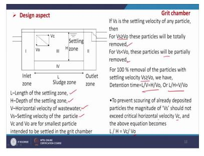
Now, we will discuss on the design aspect of grit chamber. So, grit chamber as we have discussed that the main objective is to remove the heavier particles. So, if this is a grid chamber, it has say length L and this is inlet zone, this is outlet zone. So, a particle is there, it is having two types of velocity one vertical direction velocity and other horizontal direction velocity.
