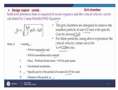
So, this is the design expression one way that we can determine the critical velocity, horizontal velocity that can be applicable for that particular grit chamber. And we can also calculate this  $V_c$  by some empirical relationship that is sufficient detention time is required to scour organics and critical velocity can be calculated by Camp-Shields Equation.
