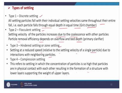
Now, we will see what are the different types of settling available in a sedimentation unit. So, one type is discrete settling that means all settling particles fall with their individual settling velocities same throughout their entire fall that is each particle falls through equal depth in equal time. So, other particles are not interfering in this case. And here good example is grit chamber where discrete settling takes place.
