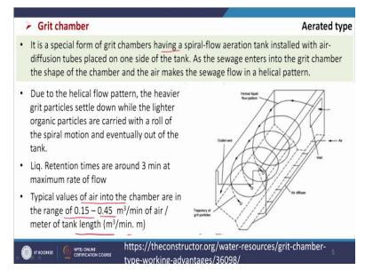
So, this type of situation will be arising, you see this is our inlet of the water and from the bottom we are giving the air. So, it is a special form of grit chambers having a spiral flow aeration tank installed with air diffusion tubes placed on one side of the tank. As the sewage enters into the grit chamber, the shape of the chamber and air mixed the sewage flow in a helical pattern, like this, it will be moving like this. So, this is a helical pattern.
