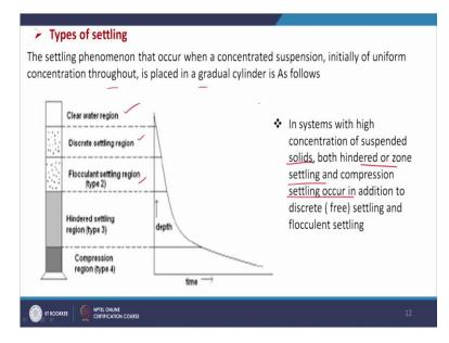
And for the more understanding of these phenomena, we can perform a simple jar test, we can take some slurry here, some solids in liquid and properly mixed. And then after a certain time we allow it to settle, we will see with time gradually the top layer will becoming to clear and the density of the layers will be varying. Initially we will be having the same but gradually it will be varying, so it will be more denser then like this.
