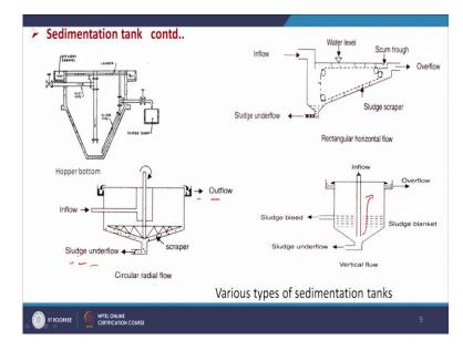
So, this is a hopper bottom tank, this is a rectangular horizontal flow tank, this is circular radial flow tank, this is vertical flow tank. So, what do we see, for this case, so what are, this is our entry and the sludge is generated here and sludge is collected here. So, this is hopper like structure the bottom part, so hopper bottom arrangement or tank.
