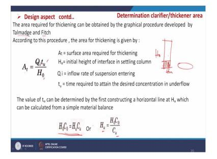
And in the thickener zone if I want to get the area requirement, then we will be doing some mass balance. So, what here we are considering that  $A_t$  is the surface area required for thickening so
