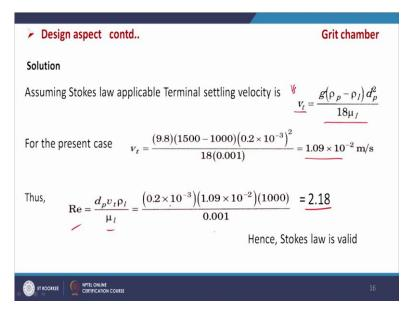
So, in this case, we can assume that the laminar flow regime is there. So, Stokes law can be applicable. So, if we apply the Stokes law we can determine the Vt terminal settling velocities that is Vs which mentioned in the previous slide that is equal to Vs, Vs, Vt same. So, g into dp minus dl into dp square by 18 mul. These expressions already we have discussed in our previous classes.
