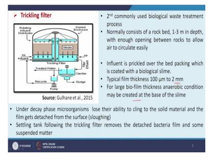
So, trickling filter as you know in this filter microbial layer is formed on some solid support and then water is passed through it and then microbes work on the organic compounds present in it and degrade it and the water is purified. So, here in this slide if we see that this is our influent here it is sprayed and this is domed enclosure and we have some media here and air influent passed here so aerobic condition is provided otherwise it will be anaerobic condition.
