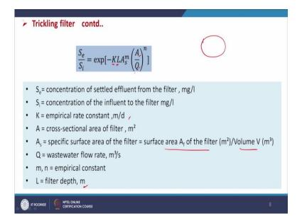
Now this case the empirical rate constant and this empirical rate constant that can be dependent on temperature and at any temperature  $K_T$
