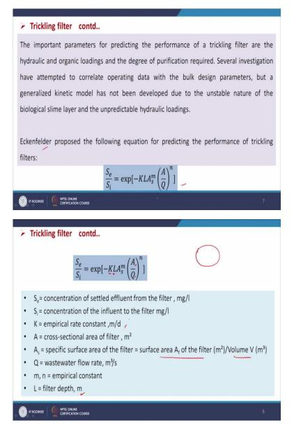
And you see here in this case, the important parameters for predicting the performance of a tinkling filter or the hydraulic and organic loadings and the degree of purification required. Several investigations have attempted to correlate operating data with the bulk design parameters, but a generalized kinetic model has not been developed due to unstable nature of the biological slime layer and unpredictable hydraulic loadings.
