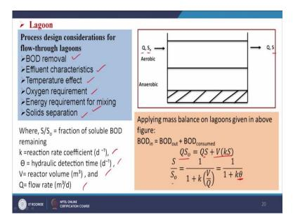
Now, we will discuss on the lagoon. So, lagoon we see that this very cheaper method for biological treatment of wastewater and here if it is a lagoon. So, Q flow rate and  $S_0$  inlet organic concentration, then S is the organic concentration in the outlet. So, in this case, if we apply the mass balance, then we will get
