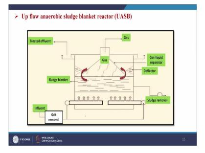
Now we will discuss on UASB that is up flow anaerobic sludge blanket reactor. So, in this case like this, so we have influent to be there and then treated effluent we will go through this and there will be some anaerobic zone and sludge blanket you will get and sludge will be collected from this and from the top gas will be collected. So this is the anaerobic sludge blanket reactor.
