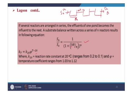
So, this is for one lagoon we are discussing, but it may happen that number of lagoons are in series, in that case, we can correlate the output and input, the outlet and inlet concentration. So, if number of lagoons in the series so, this is our inlet. So, this is our outlet, so, this outlet will be the inlet for this one. So, again this is outlet, this outlet is the inlet for this one. So, that way it will begin.
