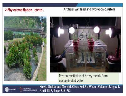
And this slide shows us some photograph, artificial wetland where the plants have been grown and used for the treatment of the wastewater and this is on lab scale setup. So, in the laboratory scale also providing control light and the plants that is Vetiveria Zizanioides have been grown here. So, for the removal of arsenic fluoride, etc. from the contaminated water.
