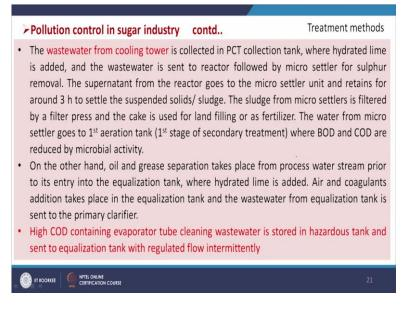
So, these are the treatment methods. So, the wastewater from cooling tower is collected in PCT collection tank where hydrate lime is added and the wastewater is sent to reactor followed by micro settler for sulfur removal. The supernatant from the reactor goes to the micro settler unit and retains for around 3 hour to settle the suspended solids or sludge. The sludge from microcellular is filtered by a filter press and a cake is used for land filling or as fertilizer.
