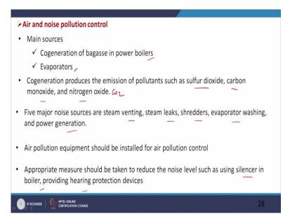
Now air and noise pollution control. So, main sources for air pollution or the cogeneration of bagasse in power boiler. So, this is the main source of air pollution and evaporators also. So, cogeneration produces the emission of pollutants such as sulfur dioxide, carbon monoxide
