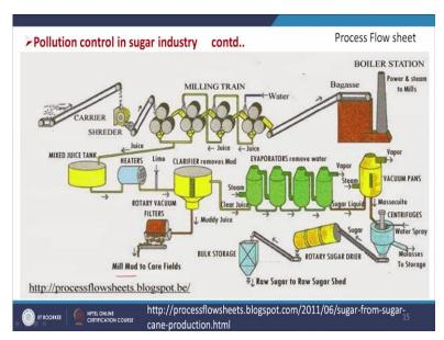
So, this is our process flow sheet for a typical sugar industry. So, here we are taking the sugarcane it is carried here. So, then it is going through the mills. So, this milling train will
