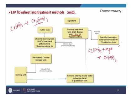
Now, we will discuss in chrome recovery part. So as you mentioned, that from the tanning unit, the chrome bearing wastewater is coming to the collection tank, then it is sent to the chrome treatment tank, where MgO magnesium oxide dosing is taking place at pH 11.5 to 12. So here we have chromium  $Cr_2(SO_4)_3$  in the solution, because chromium is here in +3 step chromium sulfate is used and which is added with magnesium oxide, so it will give us chromium hydroxide here as a precipitate.
