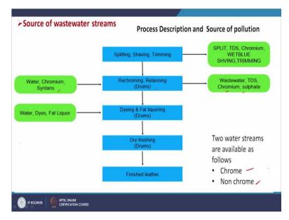
After that splitting, shaving and trimming operation takes place where we get different compositions in the water like chromium, TDS, splits, etc. And then next step is re-chroming, retanning and which takes place in drums when water, chromium and syntans are used and wastewater contains TDS, chromium, sulphate, etc.
