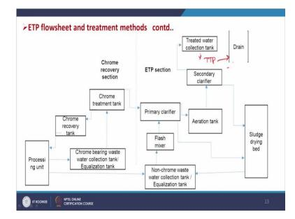
Now if this philosophy is applied, then what will happen? The wastewater which is generated that will be considered into 2 part. So processing unit if we consider this is, so it has 2 types of wastewater one chrome bearing wastewater and this wastewater is going to chrome bearing wastewater collection tank and another process water where chromium is not present, so non-chrome wastewater collection tank and equalization tank.
