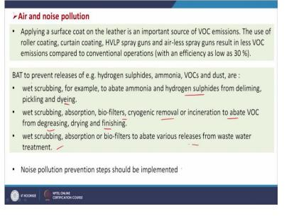
And air and noise pollution. So applying a surface coat on a leather is an important source of VOC emissions and the use of roller coating, curtain coating, HVLP spray guns and airless spray guns result in less VOC emissions compared to conventional operations. So these are some advancements in the process to reduce the VOC emission.
