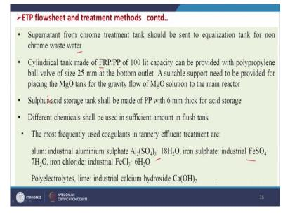
And then supernatant from the chrome treatment tanks should be sent to equalization tank for non-chrome wastewater and cylindrical tank made of FRP and PP of 100 liter capacity can be provided with polypropylene ball valve of size 25 mm at the bottom outlet. The suitable support need to be provided for fleshing the MgO tank for the gravity flow of MgO solution to the main reactor.
