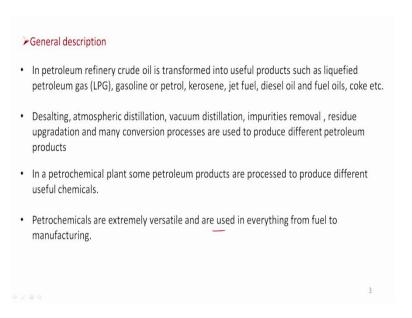
And in petrochemical plant some petroleum products are processed to produce different useful chemicals. And petrochemicals are extremely versatile and are used in everything from fuel to manufacturing different types of compounds are produced from the petrochemicals. Now, we will see the process proceed for petroleum refinery. So, overall refinery process and conversion of intermediate products. So, here we are having a crude oil, after desalting it is coming to atmospheric distillation.
