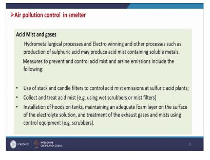
And here, if we see the air pollution, so then in air emission, acid mist, VOC particulate matter all are there. So acid mist and gases through hydrometallurgical processes and electro winning and other processes such as production of sulphuric acid may produce acid waste containing soluble metals. Measures to prevent and control acid mist and arsine emissions include the following that is use of stack and candle filters to control acid mist emissions at sulphuric acid plants.
