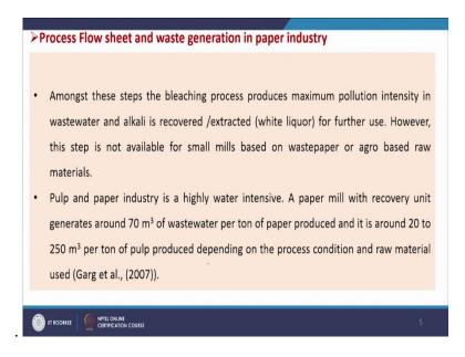
And now, if we compare the different steps through which the wastewater is generated, then you will see that bleaching process is very important where maximum pollution is generated. So, amongst these steps, the bleaching process produces maximum pollution intensity in wastewater and alkali is recovered, extracted. So, the black liquor to white liquor we get and the white liquor used for further application.
