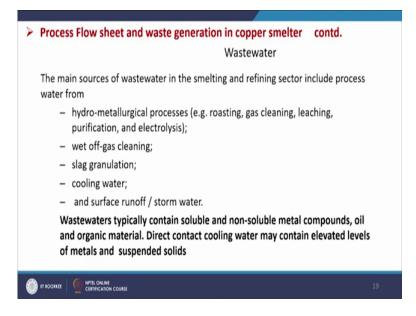
And the main sources of wastewater in the smelting and refining sector includes process water from hydrometallurgical processes, that is roasting, gas cleaning, leaching, purification and electrolysis wet off-gas cleaning, slag granulation and then cooling water and surface runoff, and stormwater. Wastewaters typically contain soluble and non-soluble metal compounds oil and organic material; direct contact cooling water may contain elevated levels of metals and suspended solids.
