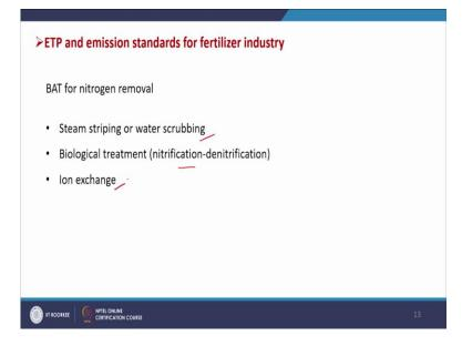
And for nitrogen removal the best available techniques are steam stripping, or water scrubbing and biological treatment nitrification-denitrification, we have discussed in case of sequential batch reactor how the nitrification-denitrification takes place also and ion exchange. So, these are the different methods that are considered at best available technique for the nitrogen removal.
