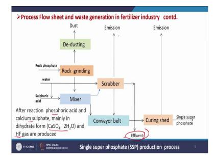
Now, we will see the process of single super phosphate production. So, SSP production, in this case rock phosphate is grinded and reacted with sulphuric acid in the mixture where this rock phosphate is converted to calcium sulphate and phosphoric acid. And mainly this calcium sulphate is in the form of  $CaSO_4 \cdot 2H_2O$  and HF gas, hydrofluoric acid is also produced.
