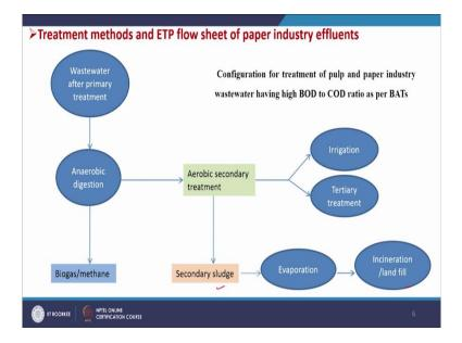
Now, you see the best available technologies, how the wastewater can be treated which are generated in this paper and pulp industry. So here wastewater certainly the primary treatment will be there. Then we will be having anaerobic digestion because COD, BOD is high. So, biogas containing methane can be produced and the slurry which is available, so that can be treated further through aerobic treatment.
