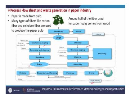
So, now, let us see first on paper and pulp industry. So, this is the flow sheet which gives the paper production. So, you see the paper making takes place basically through these two steps, one is pulping pulp production, then pulp to paper. And this pulp production is basically done from different types of fibers or many types of fibers like cotton fiber and cellulose fiber used to produce the paper pulp.
