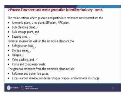
In case of NPK fertilizer. So this is a mixture so nitrogenous and phosphatic fertilizers with potassium are mixed in a reactor and then the granules are formed. So, here also different particulates emission takes place. So, now, we will see the main sections where gaseous and particulate emissions are reported.
