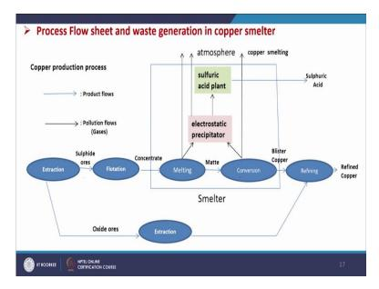
So, we know that from copper ores we get the copper and this copper may be present in ores that is oxide ores or sulphide ores. So, it is oxide ores then metal is extracted from it through hydro metallurgical processes and then if it is sulphide ores then flotation that is separated and through flotation separation or concentration takes place, then it is melted and conversion takes place and then refining it comes. So, there are two routes through which the copper is refined basically.
