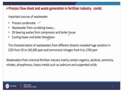
Now, we will see the important sources of wastewater. So, process condense we have seen in urea production and then wastewater from scrubbing tower, oil bearing waste from compressor and boiler house and cooling water and boiler blowdown. So, these are major source of wastewater generation. The characterization of wastewaters from different streams reveal huge variation in COD from 50 to 140,000 ppm and ammonical nitrogen from 6 to 1700 ppm.
