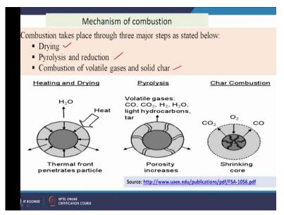
Now we will see the mechanism of combustion. So, combustion takes place through different steps. At first the drying then pyrolysis and reduction and then combustion of volatile gases and solid char. So, when we apply heat to the material in presence of oxygen, at first the drying takes place moisture goes off then the volatiles come out from the solids and then the volatiles and the residual material both are oxidized.
