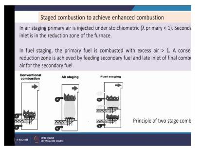
So, here we see that it is conventional combustion and here air staging. So, air is provided here primary and this is secondary air and fuel staging so here we are providing primary air and then secondary air and again we are providing the feed also.
