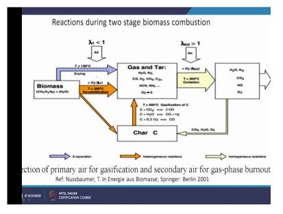
And these are the different reaction schemes so waste and biomass is coming here. So, that is first your gas and tar is produced and the remaining is your char so there will be some combustion. So, oxygen provided here  $\lambda$  less than 1 less and here secondary are more than this 1, so here there will be reactions NOx, CO<sub>2</sub>, O<sub>2</sub> will be available in excess also.
