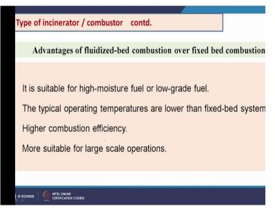
And advantage of fluidized-bed combustions are like this, that it is suitable for high moisture fuel or low-grade fuel. The typical operating temperatures are lower than fixed bed systems, higher combustion efficiency, more suitable for large scale operations.
