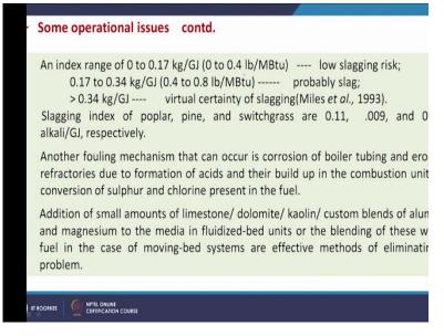
And slagging index range of 0 to 0.17 kg/GJ or 0 to 0.4 lb/MBtu, that is low slagging risk and 0.17 to 0.34 unit that is probably slag and greater than 0.34 unit that is kg/GJ that is virtual certainty of slagging. So, that will be, there is a good possibility of slagging.
