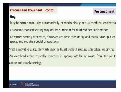
So, sorting this may be sorted manually, the MSW may be sorted manually automatically or mechanically or as a combination. There of coarse mechanical sorting may not be sufficient for fluidized bed incineration. Advanced sorting process however are time consuming and costly take up a lot of space and require special precautions with a movable grate the waste may be burnt without sorting, shredding or drying.
