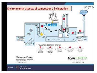
Now we will see that flue gas clean up. So, once the flue gas is generated and heat is recovered from it then steam is produced and then the flue gas is going to the environment.
