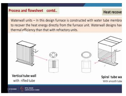
So, that is one design. Another design is there that is water wall furnace, in that case the furnace is constructed with water tube membrane walls to recover the heat energy directly from the furnace unit. So, if it is a furnace unit, in the wall of the furnace we have water tubes. So, directly it is in contact with the flue gas in the furnace itself and then water is converted to steam, so that way.
