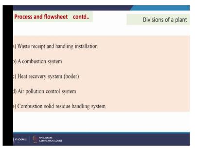
And it has different parts, this incineration plant has different parts like say waste receipt and handling installation. Then a combustion system, a heat recovery system, air pollution control systems and combustion solid residue handling system.
