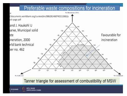
And this slide shows us the selection of the materials for incineration. So, here diagram shows that this is percentage combustible and another percentage moisture and percentages. This is favourable conditions for incineration. So, high carbon content, less moisture and less ash content are more favourable for this.
