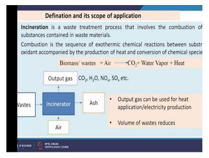
Here we will see what is incineration. So, incineration is a waste treatment process that involves the combustion of organic substances contained in waste materials. So, combustion is the sequence of exothermic chemical reactions between substrates and oxidant accompanied by the production of heat and conversion of chemical species.
