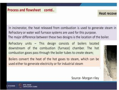
Now we are coming to heat recovery. So, heat recovery in the incinerator the heat is released and it is associated with the flue gas and that heat is used for the production of steam in boiler. So, there are two types of boiler, one is your refractory or and another is your water wall furnace systems. So, the major difference between these two designs is the location of the boiler. In some cases, we have one furnace separated by a boiler.
