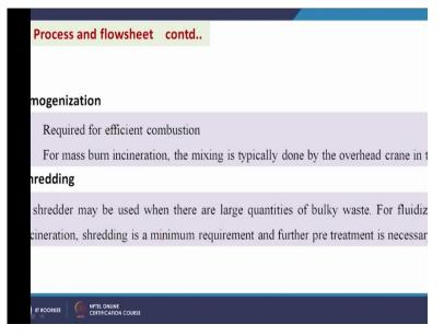
And homogenization, this is required for the efficient combustion for mass burn incineration. The mixing is typically done by overhead crane in the pit. And shredding, a shredder may be used when there are large quantities of bulky waste for fluidized wet incineration, shredding is a minimum requirement and further pre-treatment is necessary.
