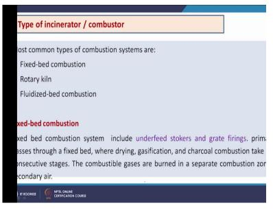
Now different types of combustion system. If we think about the reactor type, then it can be fixed-bed combustion then rotary kiln and fluidized-bed combustion. So, fixed-bed combustion in this fixed-bed combustion system it includes under feet stroker and grate firings and primary air passes through a fixed-bed where drying, gasification and charcoal combustion take place in consecutive stages. The combustible gases are burned in a separate combustion zone using secondary air.
