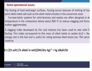
Now some operational issues we will discuss. One important issue is fouling, so why the fouling is taking place so where heat transfer is taking place in case of furnace or boiler in that case the fouling will take place. In the furnace or in the boiler, if the waste material is having very high ash content and ash is being molted in the molten stage, it is forming a slag so that will create a layer on it and the fouling will occur.
