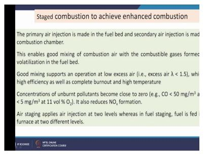
And we see that air we are providing in the first step is the primary air and the second step when we are providing it the secondary air. So, the primary air injection is made in the fuel bed and secondary air injection is made in the combustion chamber.
