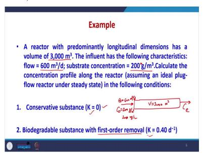
We will take example and understand this. So, a reactor with predominantly longitudinal dimension has a volume of 3000 meter cube so, it is given that a reactor is there which is having a volume of 3000 meter cube. The influent has the following characteristics. The influent which is coming to the reactor is having a following characteristic which is 600 meter cube per day is the flow rate.
