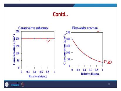
So, we can draw a figure like this the concentration in gram per meter cube remains constant and there is no mixing or nothing is happening with reactor distance whereas, the concentration decreases continuously via the first order reaction kinetics and we can see the at the exit the concentration is around 27 gram per meter cube for 5 day retention time. So, this is what is we are getting the profile is this is the profile and this is for ideal flow reactor.
