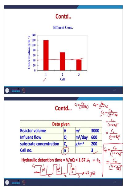
So, we use this formula for this is the d the detention time 1, 2, 3. The K values are there,  $C_0$ 's who after first cell it will be 119 then 71 then 43. So, overall, this is 78.48 which is the efficiency which is obtained and the exit concentration is 43.
