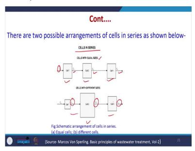
So, there are two possible arrangements of cells in series as shown below, cells with equal sizes, this is the cells in series. So, we have cell 1, cell 2, cell 3, all have equal sizes, C0 is the initial concentration and with time they are decreasing. It is also possible to have different size cells, we can see here again the concentrations are decreasing with the number of cells. So, both the conditions are possible.
