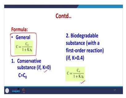
Now, for the first order we found out earlier that the equation can be written like this, the general formula is C is equal to  $C_0$  1+ $K_{th}$ . Now for the conservative pollutant K is equal to 0 so, C is equal go to  $C_0$  for biodegradable substance we will be using the same formula.
