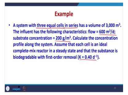
Same question which was earlier, a system with three equals cells in series now, we are assuming remember, when only one cell was there their effluent concentration was 66 when the plug flow reactor was there, the effluent concentration was 27. Now, we are assuming three equal cells in series has a volume of 3000 meter cube, the influent has following characteristics the flow rate is 600 meter cube per day, the substrate concentration is 200, the K value is 0.4 as earlier.
