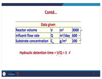
So, we have already given reactor volume, influent flow rate, the substrate concentration, the hydraulic detention time is also known to us because we have volume known to us and Q known to us. So, V by Q is 5 so, we have 5 day is the hydraulic detention time for this particular reactor.
