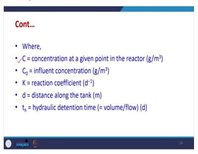
And here in this case in the previous slide, the C is the concentration at any given time in the reactor  $C_0$  is the concentration, influent concentration, which was the initial concentration, K is the reaction coefficient or the reaction constant and d is the distance along the tank which which is only true for the plug flow reactor, this the hydraulic detention time we can find out.
