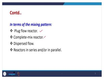
Now, in terms of mixing pattern, we can define various types of reactors and these reactors are called plug flow reactor, completely mixed reactor then we have dispersed flow reactor and then reactor in series or in parallel. So, we will be trying to learn each of them a little bit so, as to we can understand the concept and how they can be useful during the biological treatment of wastewater. So, we are going to learn them each of them in greater detail.
