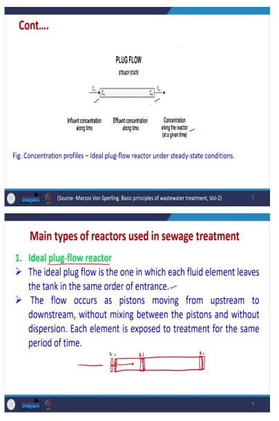
So, in this case this is the plug flow reactor, so, in this case, what we will assume that we can see here the there is a concentration  $C_0$  which is entering and  $C_e$  is the effluent concentration. So, this is the influent concentration along time. This is effluent concentration and concentration along the reactor at given time.
