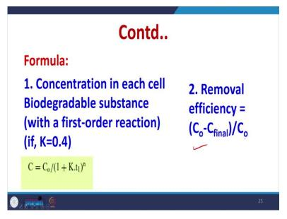
So, concentration is the each cell for biodegradable substance with first order reaction kinetics will be  $C_0$  this and overall efficiency can be  $C_0$ - $C_{final}$  / $C_0$  or  $C_0$ -C.
