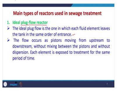
So, main types of reactor used in the sewage treatment or wastewater treatment. Firstly the ideal plug flow reactor. So, plug flow reactor that we are going to study so, ideal is the one which is same as what is the in during the ideal conditions. So, ideal plug flow is the one in which each fluid element leaves the tank in the same order of entrance. That means the fluid
