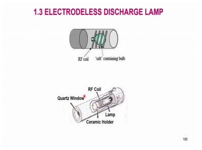
So, these are some of the problems with the material materials and they are not. So, common as a EDLs hollow cathode lamps because hollow cathode lamps are made of the same filament etcetera and they are made very easily and then it is difficult to make very few lamps are usually made of these are EDLs electrode less discharge lamps because only volatile materials need to be converted into vapor phase.
