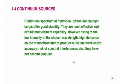
Now there are as I telling you we look at consist continuum sources. So, continuum spectrum of hydrogen xenon halogen lamps etcetera offer good stability they are cost effective and exhibit multi element capability they are; that means, you can because it is continuous several elements are detectable.
