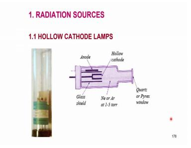
What we had discussed was about hollow cathode lamp as one of the sources of radiation which will give out the radiation of the same element which you want to determine and because the filament is made of the metal which you want to analyze the filament is in the form of a conical cylinder.
