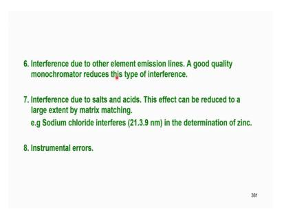
That is a good quality. Monochromator is required and other emission lines may be near by. So, if I use a filter emission will be more because there will be lot of more radiation falling on the detector. So, that is a type of interference only and then, there could be interference due to salts, acids etcetera. This effect can be reduce to a large extend by matrix matching.
