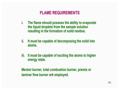
So, what are the requirements of the flame, what kind of flame we do require in flame atomic emission spectrometry? First of all, the flame should posses the ability to evaporate the liquids droplets from the sample solution resulting in the formation of the solid residue. The mechanism of this I have already given earlier and it must be capable of decompose in the solid into the atoms and it must be capable of exciting the atoms to higher energy state.
