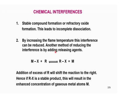
So, operation is a relative technique. Then, there could be some amount of chemical interference also. For example, some of the refractory oxide formation takes place that leads to incomplete dissociation does not melt refractory oxides, tungsten, chromium etcetera. We had discussed it earlier. So, if refractory oxide formation takes place like
