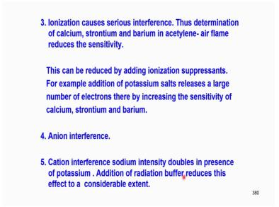
So, ionization we do not want as usual. We do not want ionization because ionization cause a series. We want atoms and we do not want ions. That is the fundamental basis of all atomic absorption spectrometry because if ions are formed, it is useless as far as emission and absorption, we want atoms in the ground state. It should go to next higher energy state and the next higher energy state atoms have to come down to the ground state by lose of energy or through the emission in with model.
