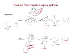
So this could be the possibility that for anti cases this hydroxy is in the other side. If you see, this is anti and hydroxy-this one is on the other side. So it cannot be coordinated chromium. So this will be less stable; less stable this one. And this will give cis, of course, and this will give the anti. So this will be trans product.
