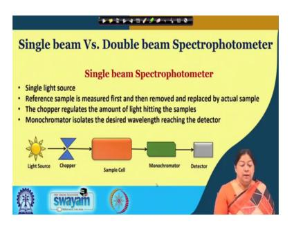
There are 2 types of spectrophotometer that are used one is a single beam one is a double beam. In a single beam case we have a sample cell and we have a reference sample what do we mean by that, if the protein is dissolved in a buffer we discussed about buffer solutions before when the protein is dissolved in a buffer, then this means that the buffer may have some components that absorb light.
