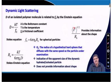
Now D of isolated polymer molecule is related to frictional coefficient by Einstein equation and this friction coefficient of rigid spherical particle is given by Stokes equation where  $R_h$  is the radial hydrodynamic radius.
