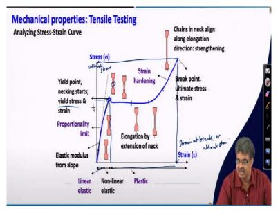
(Please refer the figure on the slide) Now this is the outcome of a tensile test - a stress-strain curve. In this case, stress is plotted in the y axis, and strain is plotted in the x axis. As I described, the sample is strained at a constant rate and the required stress is plotted in the y axis. Now in the beginning, upto a certain strain the deformation is elastic deformation that means if we leave the stress it will come back to the original shape.
