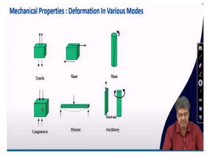
There are other possible deformations in various modes, there could be other types of shear where we are applying a circular force, if the compression is happening by applying force like this, the way it is shown this is compressive stress. This is a flexural stress where these two sides are fixed or supported and a force is applied in the middle. So it bends after applying the force like this dotted line and this is called flexural stress and this strain is called flexural strain.
