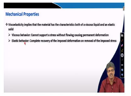
What is viscoelastic nature? Viscoelasticity implies that the material has the characteristics of both a viscous liquid and an elastic solid. Viscous behavior means that if we apply stress, I apply force to a material; it cannot resist the stress without flowing. For example, if I tilt a water bottle, water will flow; it will not be able to sustain the force, gravitation force that is acting on it. Moreover, once it flows it will be permanently deformed.
