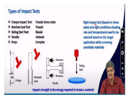
The other mechanical tests will depend on the type of material and type of application. For example, impact test is to quantify when a material face an impact like a car running hits something and then it is a sudden impact. Therefore, to test the materials' capability to resist this impact force, different types of testing are done and they are called impact test.
