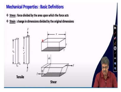
Some basic definition about mechanical properties: Stress is the force divided by the area on which the force is acting. And strain is the change in dimension divided by the original dimension. There are different types of stress like in this case a stress is applied in a longitudinal direction and this is called tensile stress and the deformation happens in a longitudinal direction or the length is increased in this case. This strain is called tensile strain.
