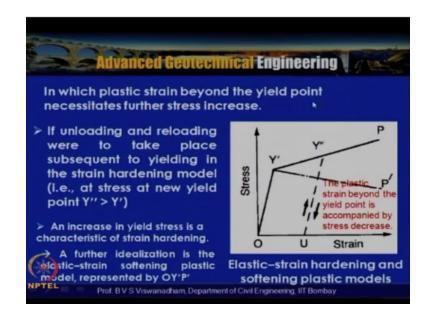
Now then, in which the plastic strain beyond the yield point and this is yet the further stress increase. So if unloading and this is particularly elastic strain hardening and softening plastic models. That means that sometimes beyond, you know the yield point there can be hardening or there can be softening, you can see that in increase in the stress or decrease in the stress.
