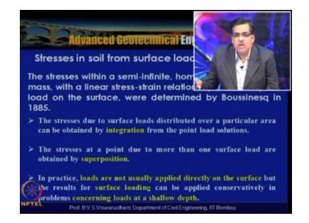
So the stresses within a semi-infinite, homogenous, isotropic mass, with a linear stress strain relationship, due to a point load on the surface, were determined by Boussinesq in 1885. The stresses due to surface loads distributed over a particular area can be obtained by integration from the point load solutions. And the stresses at point due to more than one surface load are obtained by superposition.
