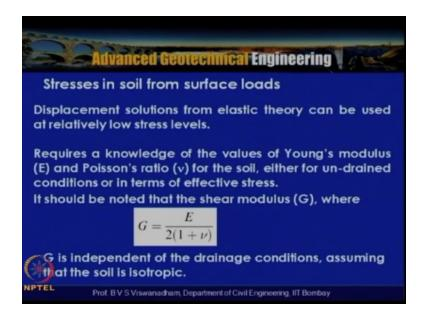
So displacement solutions from elastic theory can be used at relatively low stress levels. Requires a knowledge of the values of Young's modulus E and Poisson's ratio v for the soil, either for un-drained conditions or in terms of effective stress. It should be noted that shear modulus G, where G=E/2(1+v), G is independent of the drainage conditions, assuming that the soil is isotropic.
