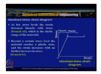
If you look into the idealized the stress-strain diagram, in this particular slide the idealized stressstrain diagram is shown here. The stress is on the vertical axis and strain on the X-axis. And the zone AB is in the elastic range and zone BC is idealized as plastic. So you can see that at low stress levels the strain increases linearly with stress and that is the branch AB, which is elastic range of the material.
