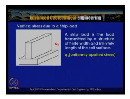
A here strip load is the load transmitted by a structure a finite with of infinite length of the soil surface, so before looking into this let us try to look into the problem with one second with how to construct a stress isobar for you know if the point load is about 2000KN so let us look into this particular problem.
