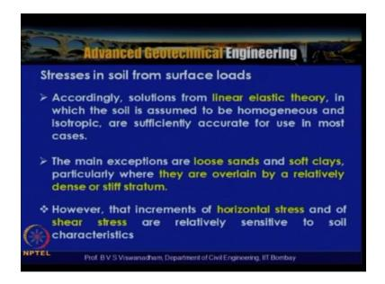
So accordingly the solutions from linear elastic theory in which the soil is assumed to be homogenous and isotropic, and are sufficiently accurate for use in most cases. And the main exceptions are loose sands and soft clays, particularly where they are overlain by a relatively dense or stiff stratum. Then, you know this is some of the exceptions which are followed. However, that increments of horizontal stress and of shear stress are relatively sensitive to soil characteristics.
