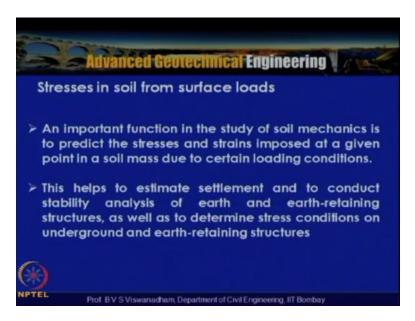
So always the surface is actually subjected to loading, so in that case an important function is the, in the study of soil mechanics is to predict the stresses and strains imposed at a given point in a soil mass due to certain loading conditions. Basically this helps to estimate the settlement and to conduct the stability analysis of earth and earth-retaining structures. As well as to determine the stress conditions on underground and earth-retaining structures.
