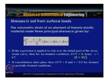
And particularly we are now talking about the volumetric strain of an element of linearly elastic material under three principle stresses is given by  $\Delta v/v=1-2 v/E(\Delta\sigma 1+\Delta\sigma 2+\Delta\sigma 3)$ . If this expression is applied to soil is for the initial part of the stress strain curve, then for un-drained conditions the  $\Delta v/v=0$ , and once you put  $\Delta v/v=0$  with v=0.5 then for un-drained conditions E=3 times G that is the G is nothing but E/3.
