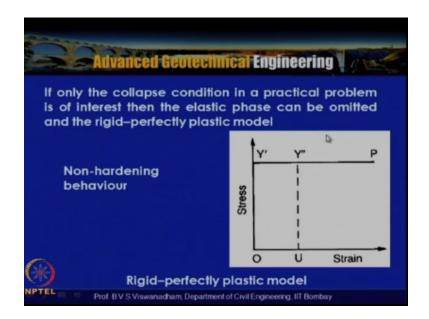
If only collapse condition in a practical problem is of interest, then the elastic phase can be omitted and rigid-plastic model, rigid-perfectly plastic model can be assumed. So that means that the linear elastic segment is ignored, then directly we have taken the OY' and Y'P. So this is nothing, but a non-hardening behavior and rigid-perfectly plastic, this is this trusted relationship is indicated as rigid-perfectly plastic, that is OY' and Y'P.
