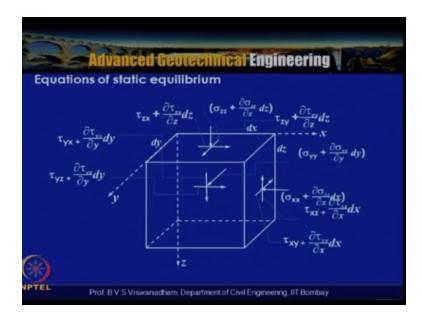
Now let us look into deducing the equation of static equilibrium. So consider the same stresses which are actually acting in X axis and Y axis and Z axis. And we have bought, there is a increase in the stress because of the self weight of the element. So we have on the X axis  $\sigma xx$  which is acting and the other phase which is actually having  $\sigma xx + \partial x(dx)$  and on the Z axis it is  $\sigma zz + \partial \sigma z/\partial z$  and dz.
