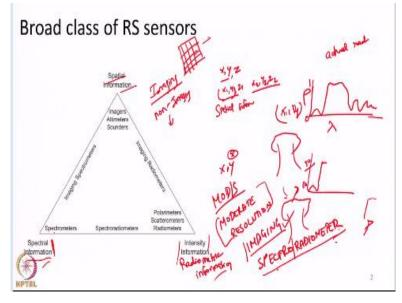
So, any remote sensing sensor can collect spatial information, spectral information and intensity information. Intensity information, we can also call it as radiometric information. Spatial information is data about any given ground point x, y. Say, for example, if I collect the elevation of all ground point x 1, y 1, z 1, x 2, y 2, z 2. if I collect such data at a given ground point, ground coordinate x, y, what is the elevation of the point?
