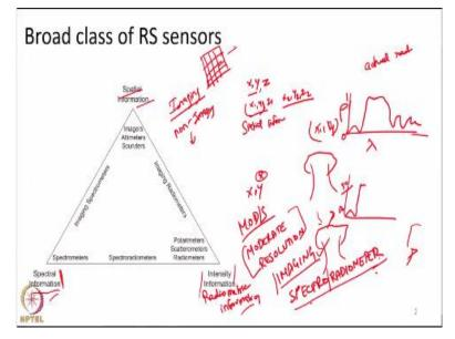
In the last class, we discussed briefly about the different types of remote sensing sensors which collects spatial information, spectral information and radiometric information. I also told you some of the most commonly used satellites from which we are acquiring data such as Landsat or MODIS, etcetera. They collect all sorts of information; they collect spatially; they collect spectral information and also they collect radiometric information.
