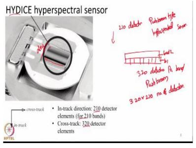
Now, this slide shows an example of an hyperspectral sensor. Where it will be like in the along track direction, there are 210 detector elements, in along track like this. So, there are 210 detector elements. In the across track, we have 320 detector elements. So, that is each band has 320 detectors, 320 detectors per band. Essentially, this is a Pushbroom type of sensor and for each band, there will be one row detector.
