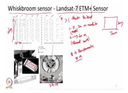
So, we will see few examples of such scanner sensor, scanning elements or hyperspectral array elements and so on. So, if you look at this particular slide, here we are showing the sensor or detector arrangement for a sensor known as Landsat 7 ETM plus. Landsat 7 is the name of satellite, this is the name of the sensor enhanced Thematic Mapper plus. It was a Whiskbroom scanner.
