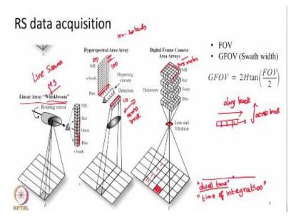
In this figure what is shown is Whiskbroom scanner. So, what exactly is the Whiskbroom scanner? Let us assume that data is being collected in 4 different bands blue, green, red and NIR but instead of having just one detector element per band, now we are having 4 detectors elements per band. So, this 4 is for blue, the next 4 is for green, again it is for red like that.
