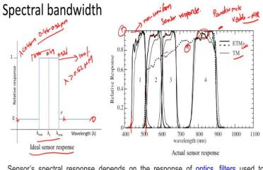
Sensor's spectral response depends on the response of optics, filters used to separate wavelengths and the detector used to collect the radiation.
