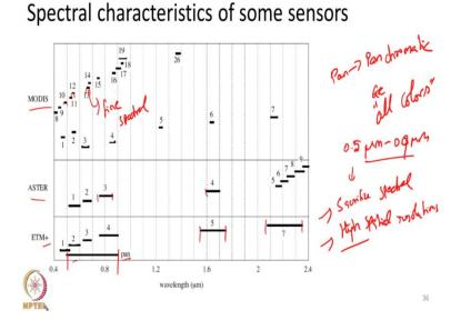
So, this line gives you spectral characteristics of some sensors. This is ETM+ sensor, ASTER sensor, MODIS sensor and so on. So, here you can see what is known as a pan band written as pan, which is panchromatic. So, panchromatic generally means all colors chroma means colour. So, essentially panchromatic band spans a very large bandwidth. Spectral resolution maybe here 0.5 to 0.9 micrometers.
