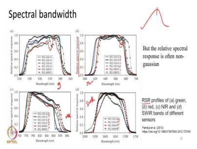
The sensor names are listed here, primarily they are launched by ISRO. So, we can see from this. the spectral response of sensor is not even close to Gaussian. Instead of having one single peak, we have a flat curve here, a high amount of variation here, a long tail here and so on.
