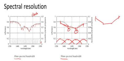
The location of central wavelength and the spectral bandwidth affects the radiance we collect from the earth's surface.
