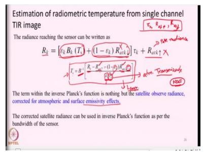
So, here in this particular slide this is the equation we used for the retrieval of LST. So, the inverse Planck's function of the radiance received at the sensor after being corrected for atmospheric effect and surface emissivity effect.
