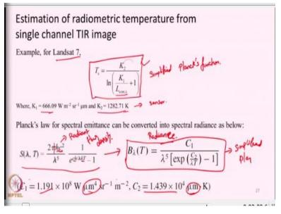
And atmospheric correction tool we have already seen. And if we substitute all the values, if we correct that satellite observed radiance and substitute in the simplified Planck's function. This is specific for Landsat sensor, this constants K 1 and K 2, these will vary for sensor to sensor. So, this equation is specifically for Landsat satellite with the corresponding K values for Landsat 7.
