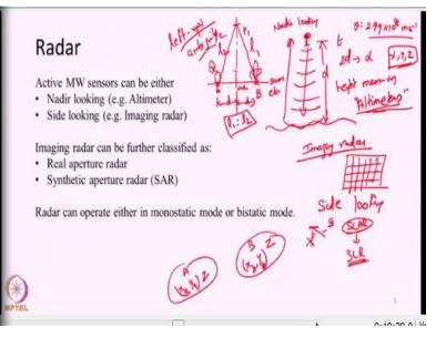
So, a radar is basically a sensor which will transmit microwaves. Here even though the acronym stands for radio detection and ranging, initially when it was formed, it was formed with respect to radio waves which is as much longer wavelengths. So, we have a system which will produce electromagnetic radiation with a given frequency and that will transmit the electromagnetic radiation, then it will receive the signal back.
