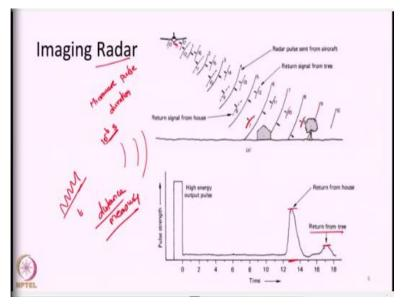
So, this is the aircraft in which the radar is mounted, the antenna is looking like this. So, this will transmit a microwave pulse, we call it as pulse for a certain duration of time, that is let us say  $10^{-6}$  seconds. So, this will transmit some electromagnetic radiation for certain length of time. For a time period of T it will be transmitted, so there will be one pulse in the air.
