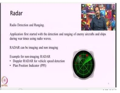
So, what exactly is active microwave remote sensing? In active microwave remote sensing what we are going to discuss is the imaging radar. So, what exactly radar is? Radar is an acronym that stands for radio detection and ranging. So, in the earlier days, during world war times, this particular technology was used for surveillance of incoming enemy aircrafts. That is, microwave transmitters will be fitted along the borders and they will be transmitting radar pulses continuously.
