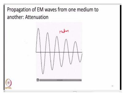
So, this is like a schematic representation of attenuation. Like some medium is present here, when EMR passes through a medium its amplitude will be going down. And finally it may also be totally absorbed within the medium. So, its amplitude will be reducing and hence its total energy content will be reducing.
