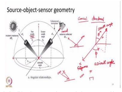
Here in this particular slide, what we are going to see is, how a source-object-sensor geometry affects our measurement. Please look at this particular thing. This is an object on the earth's surface and that will be irradiated by sun. We call it as irradiation on the object because sun energy is coming and falling on it. As I said, truly speaking, sun's energy should be considered as conical.
