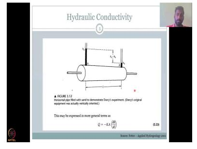
Moving on, we have a horizontal pipe filled with sand to demonstrate Darcy's experiment in a different book I have taken a different approach to just show the same explanation, but in a more different way, then the Darcy's book. So, horizontal pipe filled with sand, so, there it was slanting, but here it is an horizontal pipe to demonstrate Darcy's experiment. So, as the book says it is originally vertically or slanted position but we can also expend it in a horizontal way.
