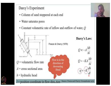
This slide, so, in the Darcy's experiment what we noticed is that the column of sand stoppered at each end so, either sand, soil, rocks materials, the material the matrix is kept in a tube and it is stoppered, a rubber stopper is put on the top and bottom. Water saturates the pores; water is fully saturated inside the pore space. Now apply yourself to the previous lectures, if we say porous space is fully filled with water that means it is a saturated system.
