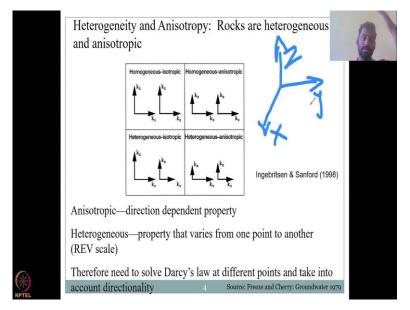
Not only this, so, why was the range present and also what are the differences in the hydraulic conductivity? Let us look at a typical case. So, we have a high heterogeneity in the system and anisotropy in the system. When I say system it is the soil or the rock matrix. Rocks are heterogeneous and anisotropic same with soils. Let us see what does that mean? What does the, what do you mean by heterogeneity and anisotropy.
