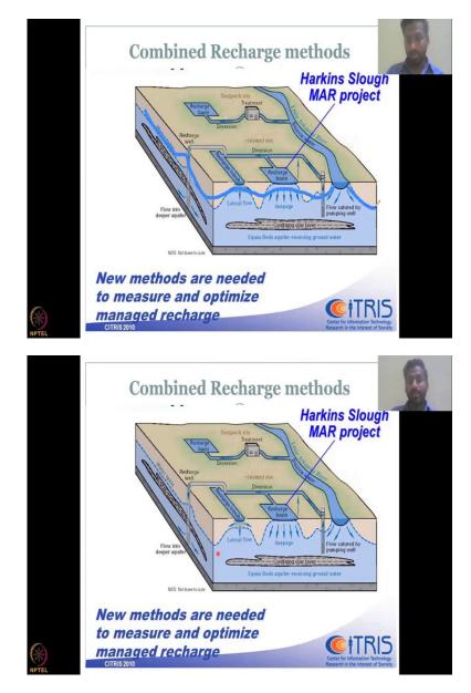
If you look at this land, this piece of land where you have a lot of water which is coming and it is been treated and put into recharge basins, which is a part of a direct method. And then you also have a recharge induced well, which is pushing the water in. So what you are seeing here is a combination of multiple method because, one method may not be just enough for your activities.
