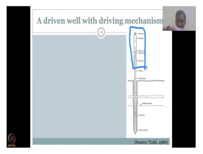
Now, how can you hit it? You can hit by a hammer mechanism but you have to be careful not to put weight on one side because the cap will go given or the drive point will turn. So, this has to be straight as much as possible for which there is a hitting mechanism, proceed here, it is just a weight you pull and then drop. You pull the weight on and then drop it will just hit, hit, hit and then it goes very very slow.
