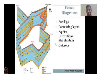
So, now we have seen more examples, it is called either Fence diagrams, you will see the word fence diagrams because you are creating a fence using the borelogs and in between you are connecting all the logs. I will again come back to this Khan et al paper in the next class because we can look at how do you read in between the fence diagrams and also discuss about borelogs connecting layers for disposition stratification and outcrops. I will see you in the next class thank you.
