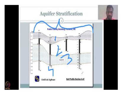
Let us take a very simplified example, one more example, so you have B1, B2, B4 and B3, again the numbering is up to you, you should pick the numbering and you have four wells, how many layers do we have one layer, two layer, three layer and four layers. At the max four layers and here you have only three layers and this one has two layers, actually this one also has a four layer, so this one has two layers.
